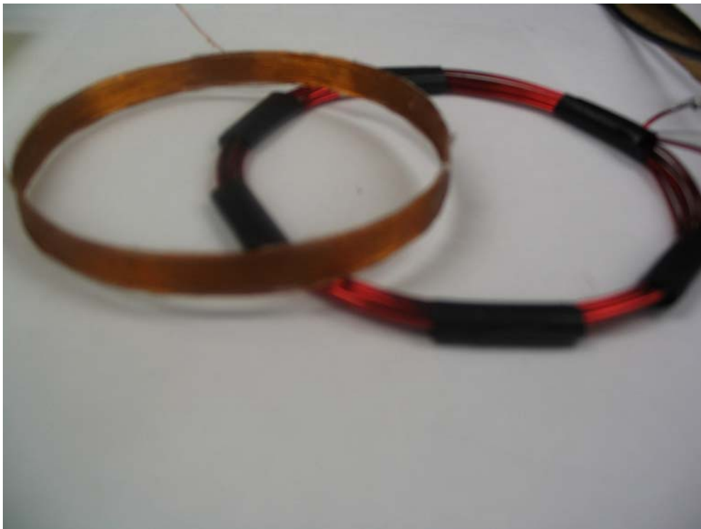
Figure 5.8 Primary (on the right) and secondary coils
