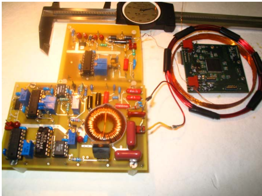
Figure 5.10 External and internal RF units, the inductive link (coils) and the perfusion sensor system's electronic interface (within the circumference of the secondary coil)
