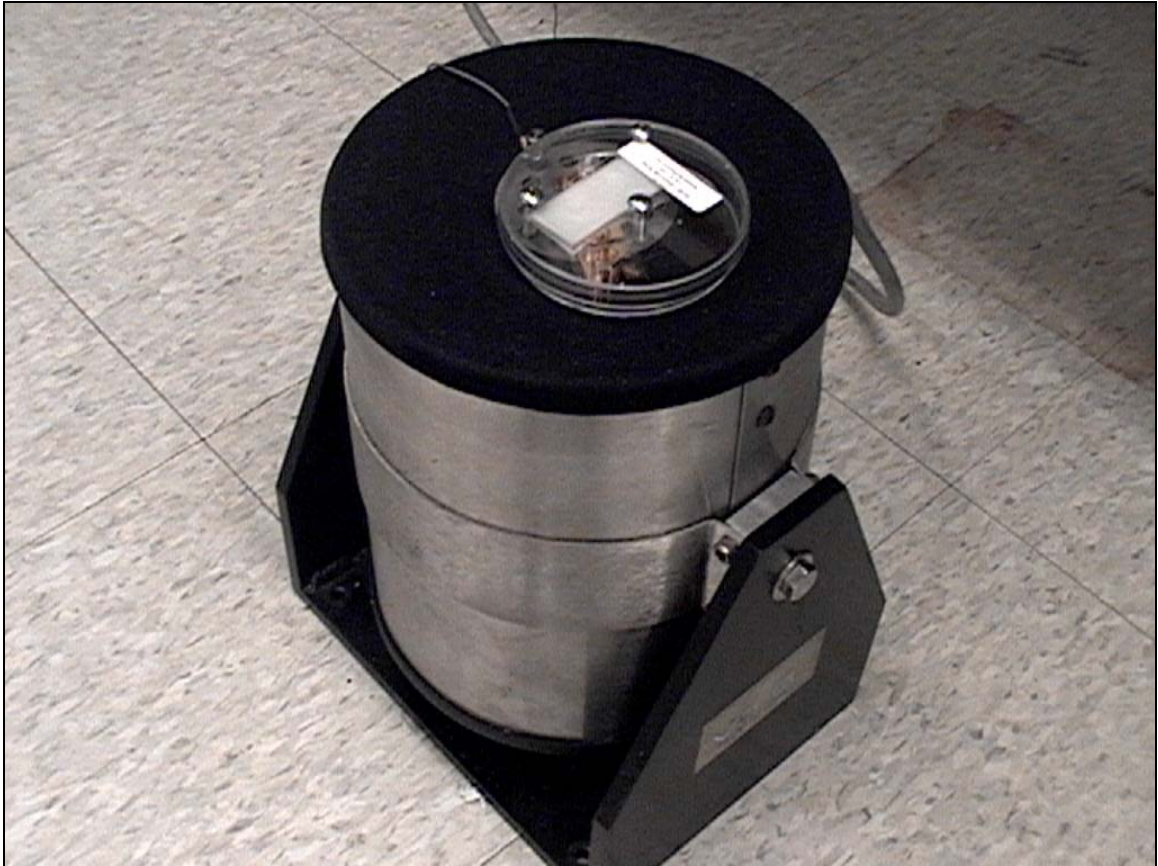
Figure A-33. Shaker used to induce vibration in the PPAEC monolayers contained in the 5 well ECIS array.
