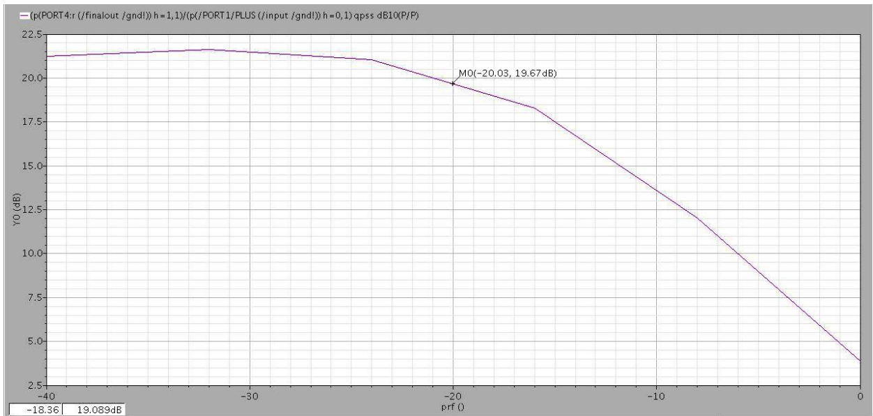
Figure 4.14 Power gain of the complete circuit
