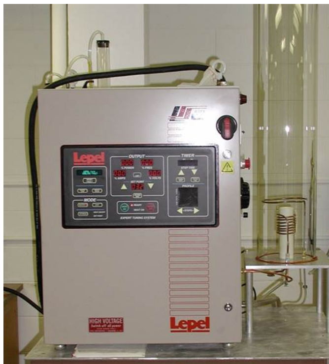
Figure 1.3: Image of the synthesis apparatus. The Lepel RF generator supplies power to the coil which inductively heats the graphite crucible and contents. Not shown are the gas tanks of argon and oxygen which are situated behind the generator.
