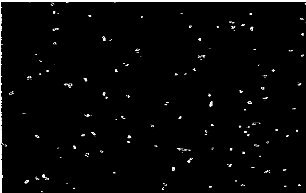
Figure A3-29. Image after the Dilation method which fills the holes formed during the edge detection method.
