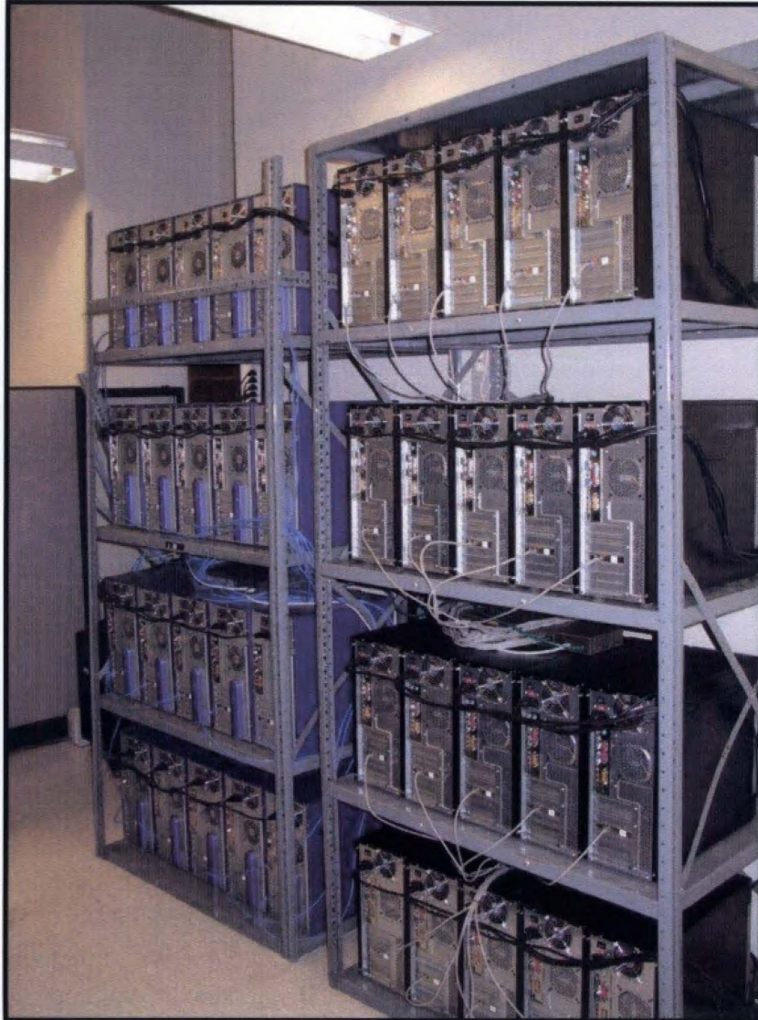
Figure 3.3: The full rack of 40 compute nodes that make up the 80 CPU cluster consist of machines based on Athlon MP 2000+ (left) and Athlon MP 2400+ (right) CPUs. Two network switches are located above the second level of nodes. The nodes are mounted facing the rear of the rack in order to facilitate access to the network and power connections and to exhaust waste heat into the center of the room.
