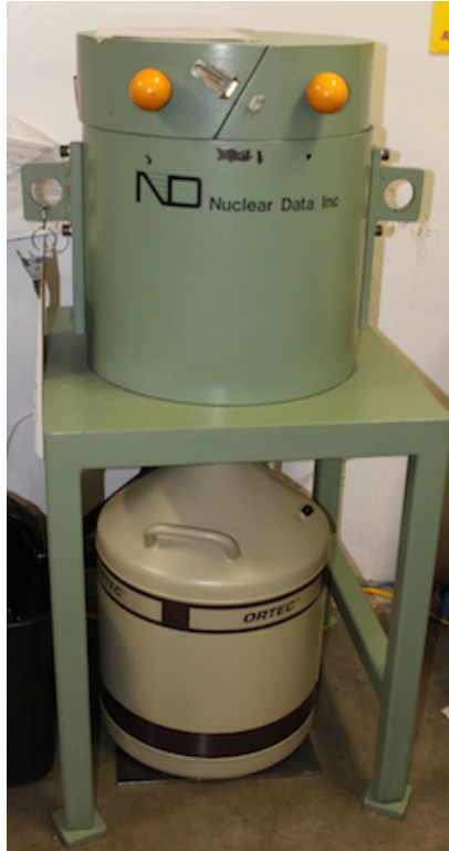
Figure 3.3: Graded lead shield with copper liner above the 30 L LN 2 dewar.
