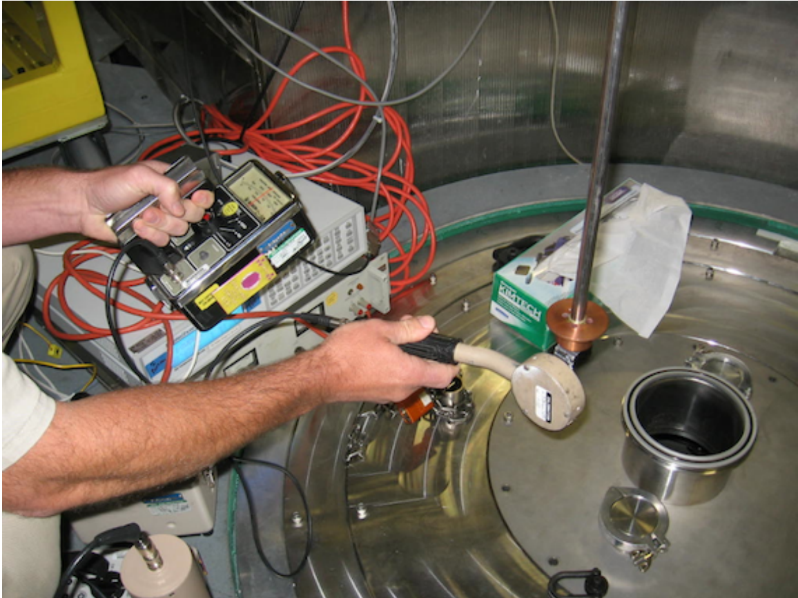
Figure 5.3: Radiation control technician checks the dose rate on the foils as they are removed the sample position after irradiation.
