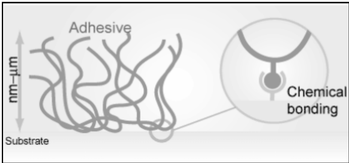
Figure 2.4: Chemical bonding of adhesive and substrate [4].
