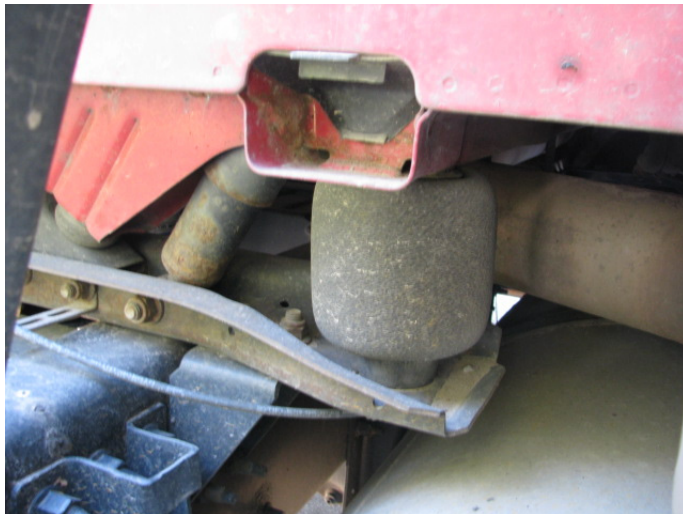
Figure 5-2 Cab spring-damper from manufacturer producing significantly lower vibrations
