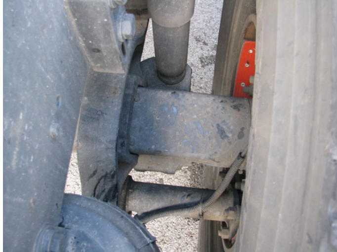
Figure 5-4 Recommended transducer placement on axle
