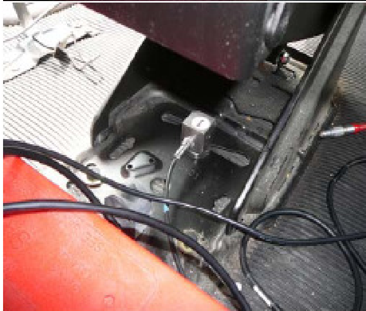
Figure 3-2 Tri-axial accelerometer underneath driver seat
