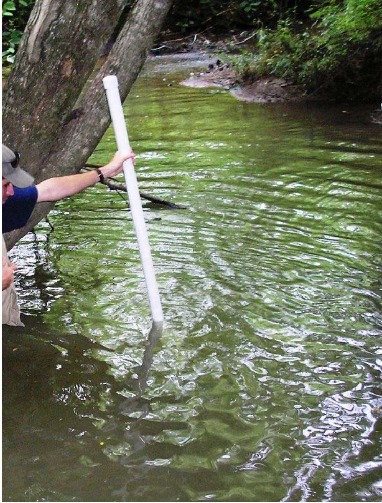
Figure 5. Maximum pool depth measurement taken in the thalweg. June 24, 2005; Site 11, Grassy Creek.
