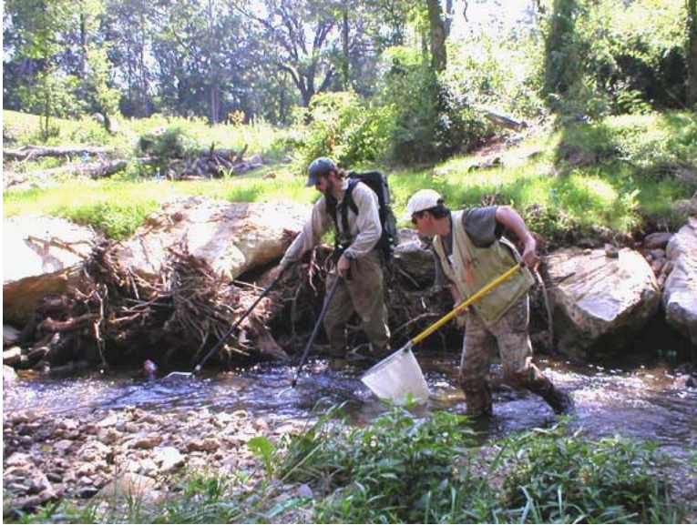
Figure 7: Depicts the use of a backpack shocker. This device stuns fish that are either immediately netted or swept to a downstream seine net. June 22, 2005; Site 11, Williams Creek.
