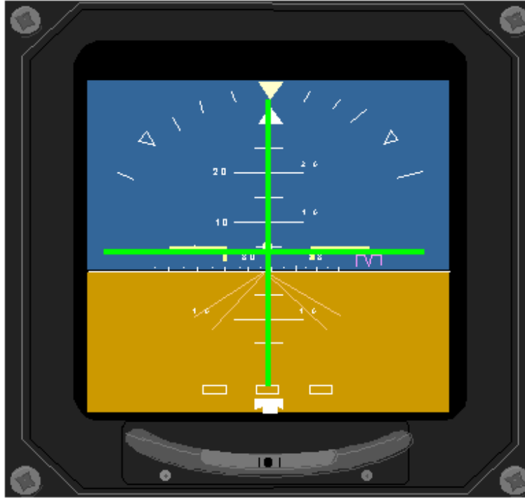
Figure 24: EADI ILS MODE WITH NEEDLES
