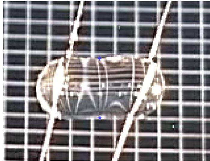
Figure 31: Image of Strings Holding Droplets Apart and Effecting Viscosity Measurements
