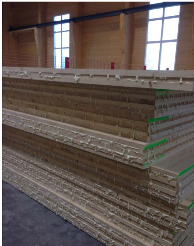
Figure 31: CLT panels after surface bonding with adhesive residues and unleveled edges. Courtesy of Dr. Timothy M. Young
