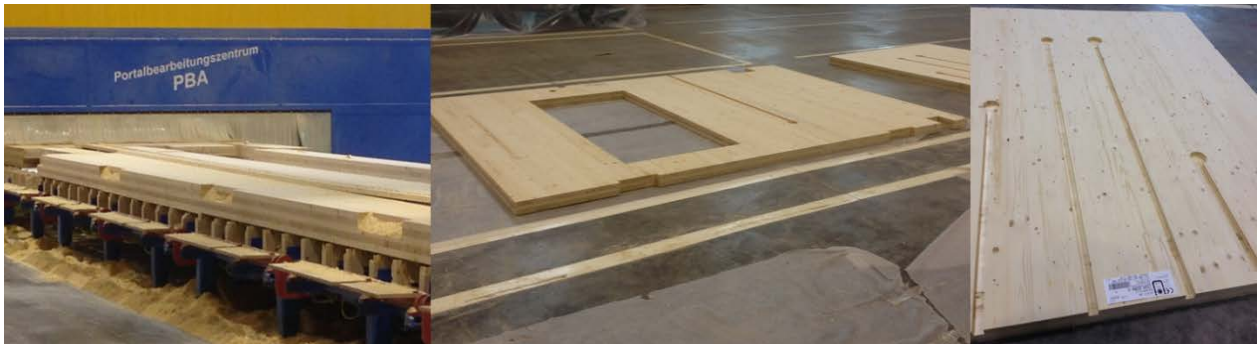
Figure 35: Finished panels after multiple processing center. Courtesy of Dr. Timothy M. Young
