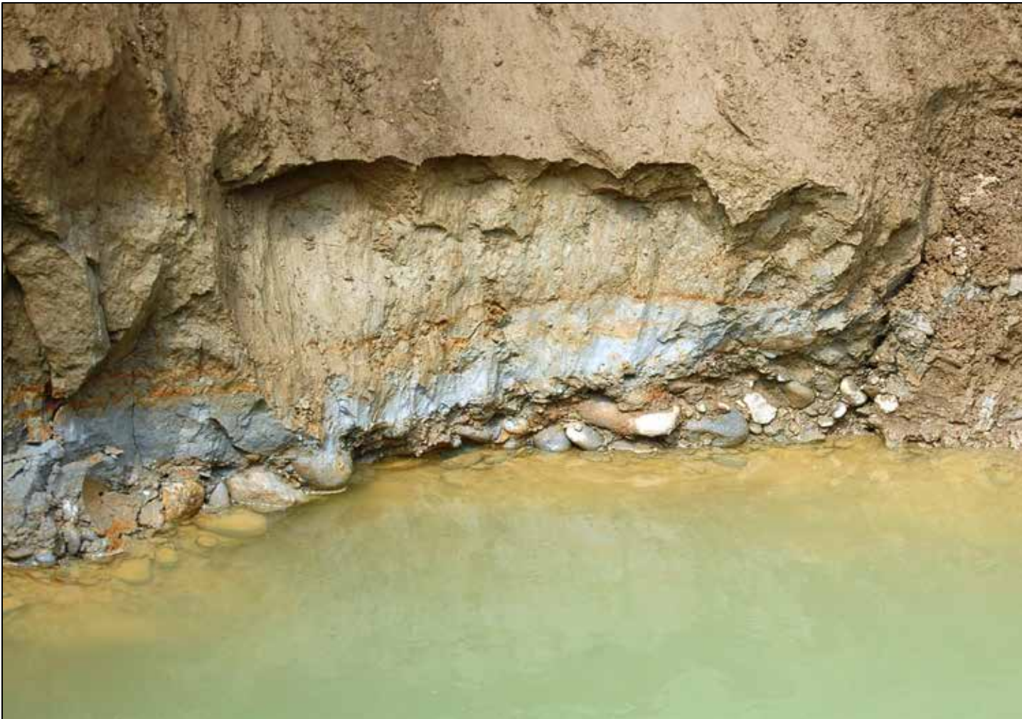
Figure 3.17 – Alluvial sediments with gravel, cobbles and boulder size alluvial deposits just above the bedrock in the sinkhole excavation.
