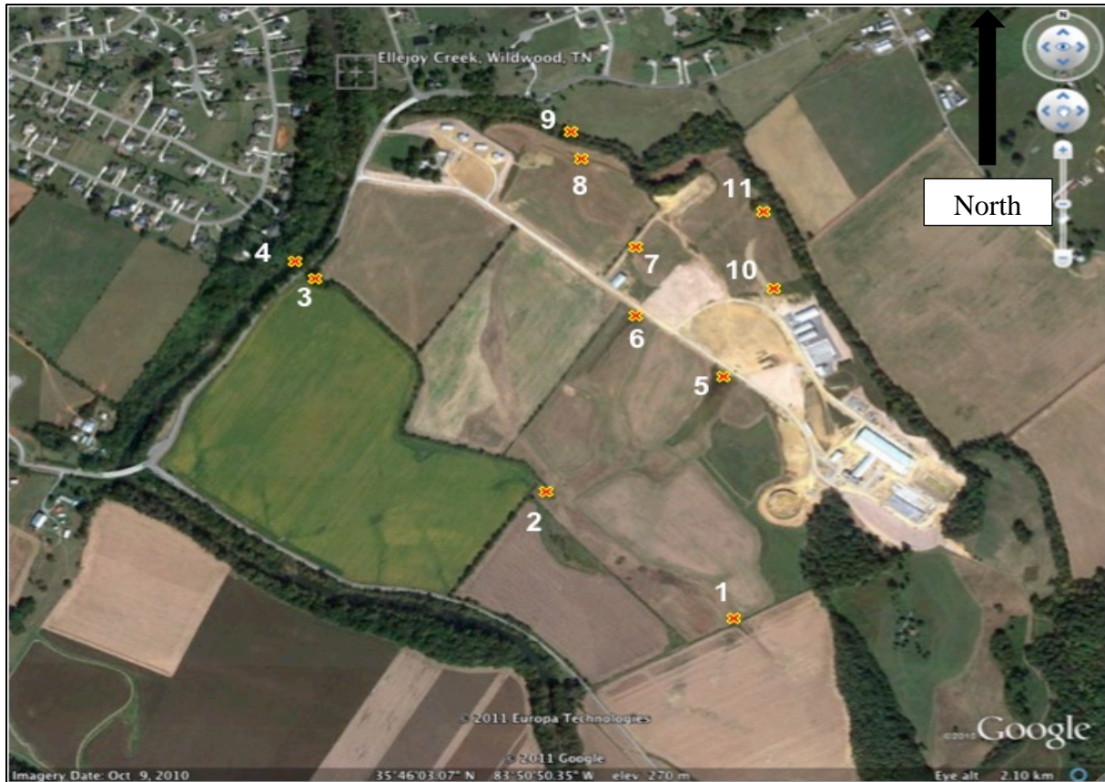
Figure 2.9 - Stormwater runoff sampling locations. Site 1 A&B: culverts source from adjacent property; Site 2, Weir; Site 3, Weir; Site 4, Little River; Site 5, Wetland before entering culvert; Site 6, Wetland before entering culvert; Site 7, Before gravel road; Site 8: Flume, Site 9: Ellejoy Creek, Site 10: Below headwall, Site 11: just before outlet to Ellejoy Creek. (Ludwig, 2011). Note: Dr. Ludwig's monitoring program uses some of the same sampling locations as the previous surface water monitoring program (Figure 2.6) but uses different designations for the sites.
