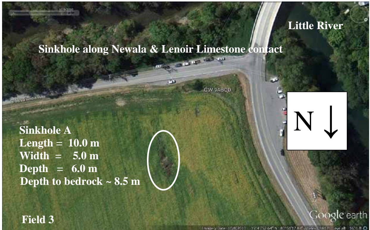
Figure 3.5 – Sinkhole (A) activity Field 3 Little River Dairy Farm. During 2010 -2012 the sinkhole expanded from 3.6 X 4.5 X 2.0 meters (L X W X D) to 9.0 X 9.0 X 5.5 meters. In late 2012, this sinkhole series was excavated to bedrock, lined with a geotextile liner and filled with rip-rap which included progressively smaller stone sizes (See Figure 3.6) (Image 10-8-2010 Google earth®).
