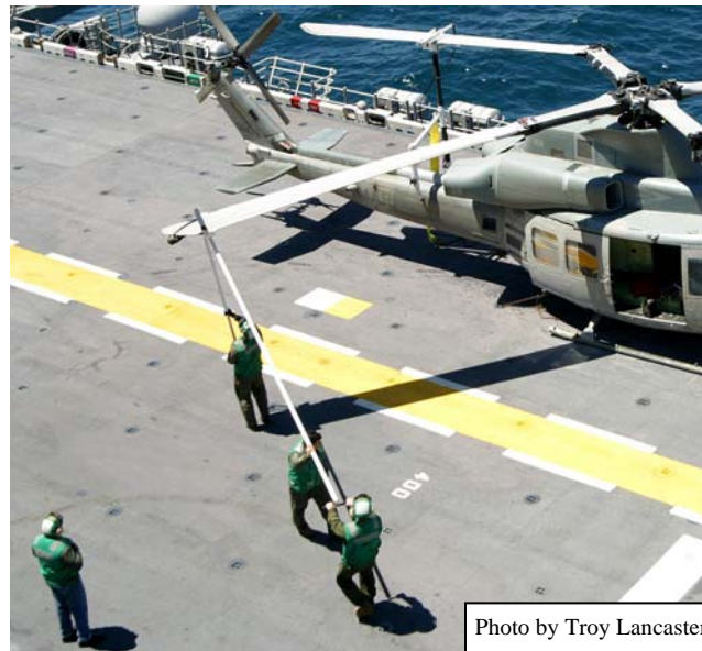
FIGURE 10: BLADE SUPPORT POLE AND BLADE HANDLING POLE IN USE
