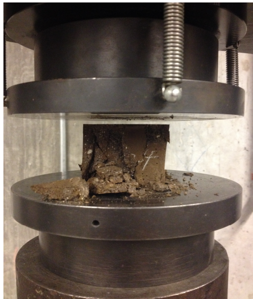
Figure 3.3 Completed USC test on Type II CEAM.
