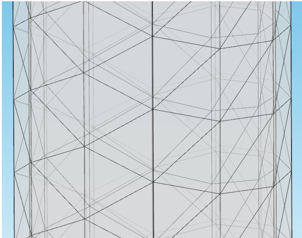
Figure 12. Blown-up view of the heat exchanger mesh in the tube walls.
