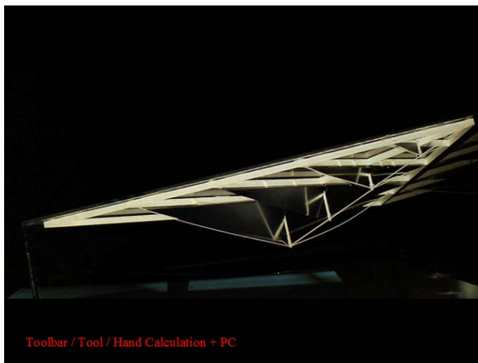
Figure 309. Scale model of light wings in one Light Prism in scale 1:10. Photo Pekka Salminen Architects
