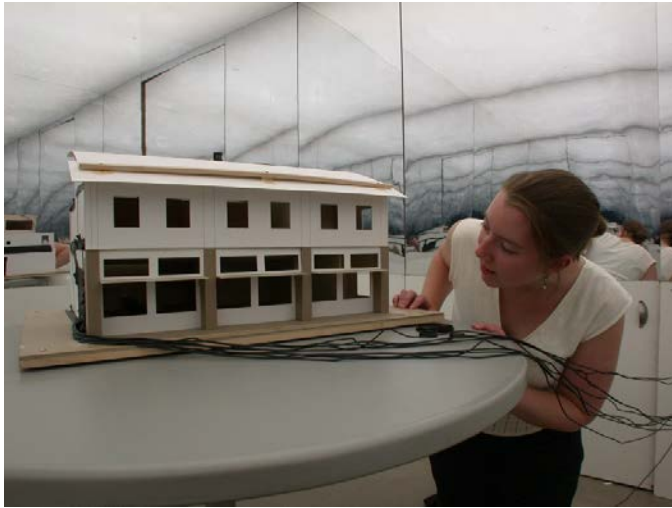
Figure 7. Daylight study at PEC lab
