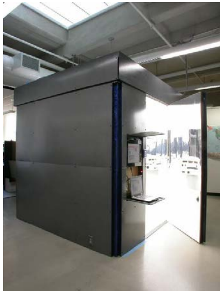
Figure 5. Overcast Sky Simulator. Photo Pacific Energy Center
