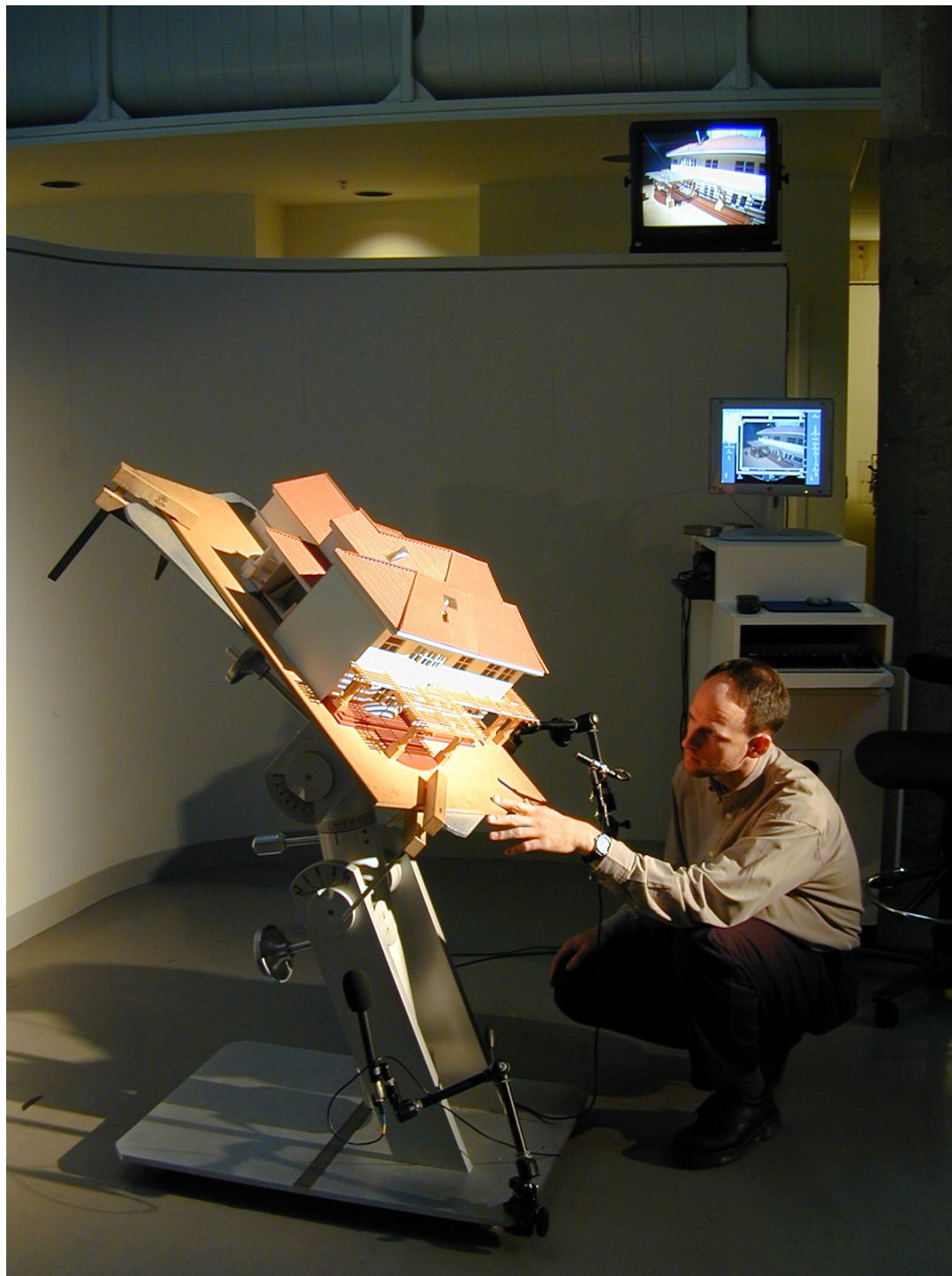
Figure 266. Heliodon in use. Photo PEC
