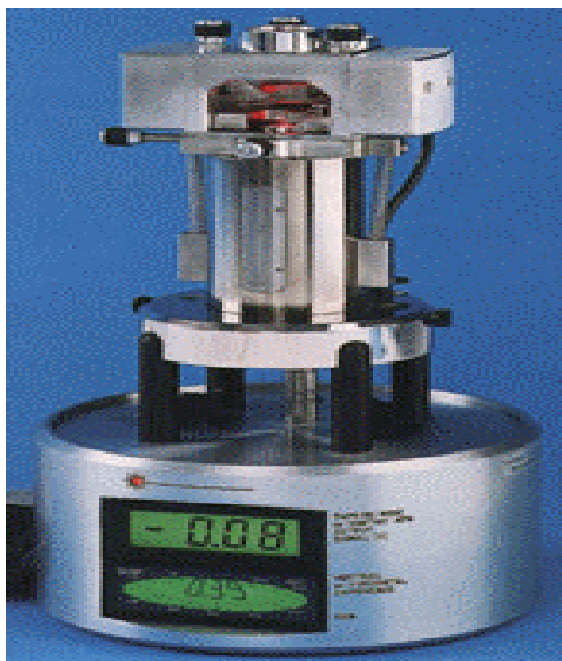
Figure 1: Digital Instruments Multimode™ AFM optimized for high-resolution force measurements and topographic imaging [9].
