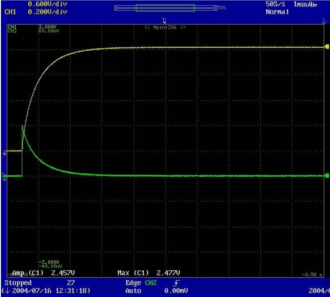
Figure A1.2-1: Oscilloscope Screen Capture of 50 A Charge Cycle at T= -25°C (Timescale: 1 min/div)
