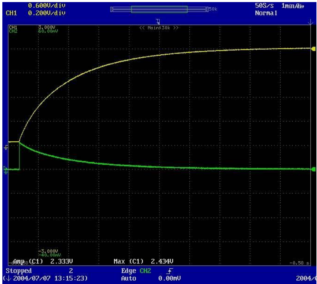
Figure A2.1-9: Oscilloscope Screen Capture of 25 A Charge Cycle at T= 25°C (Timescale: 1 min/div)
