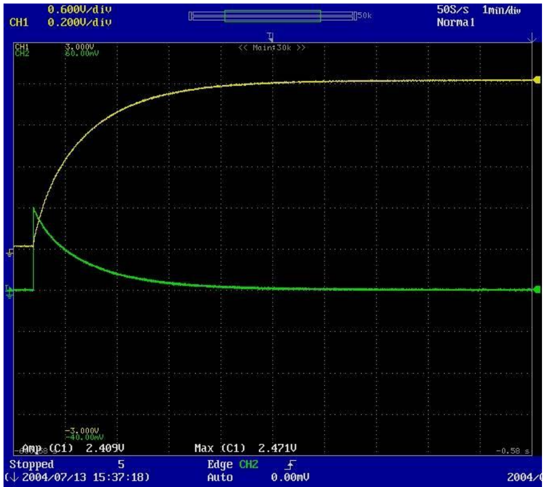
Figure A2-2-5: Oscilloscope Screen Capture of 50 A Charge Cycle at T = 0^{\circ}\text{C} (Timescale: 1 min/div)
