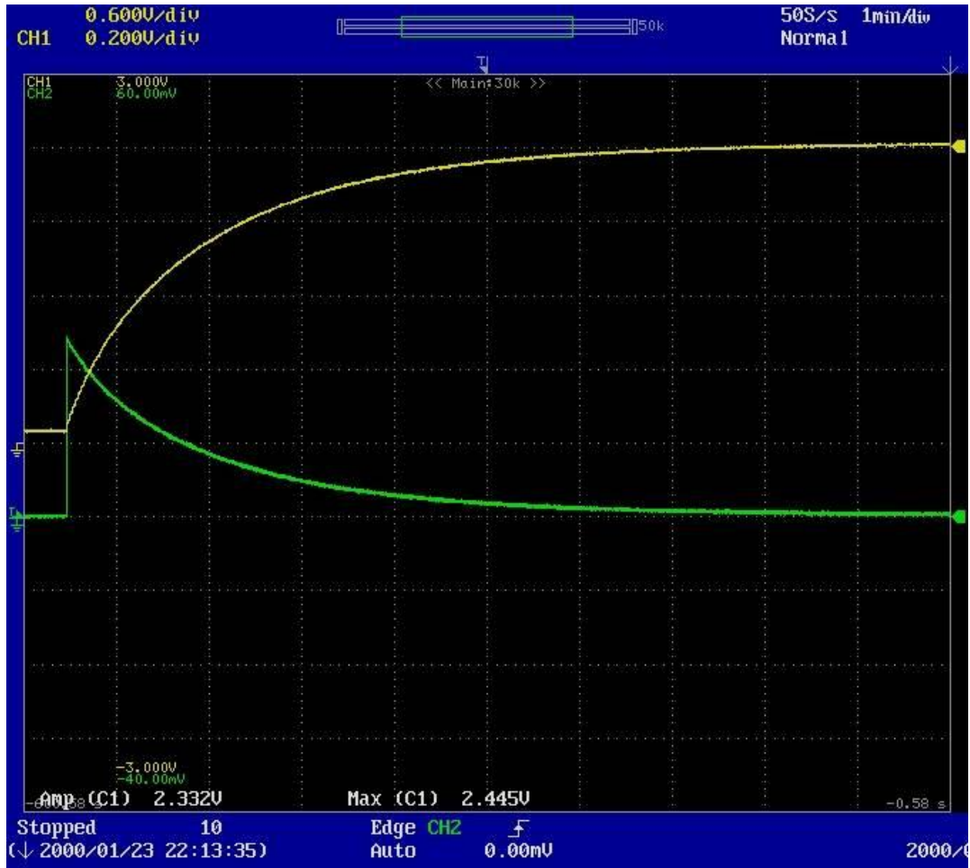
Figure A3.3-9: Oscilloscope Screen Capture of 60 A Charge Cycle at T = 25^{\circ}\text{C} (Timescale: 1 min/div)
