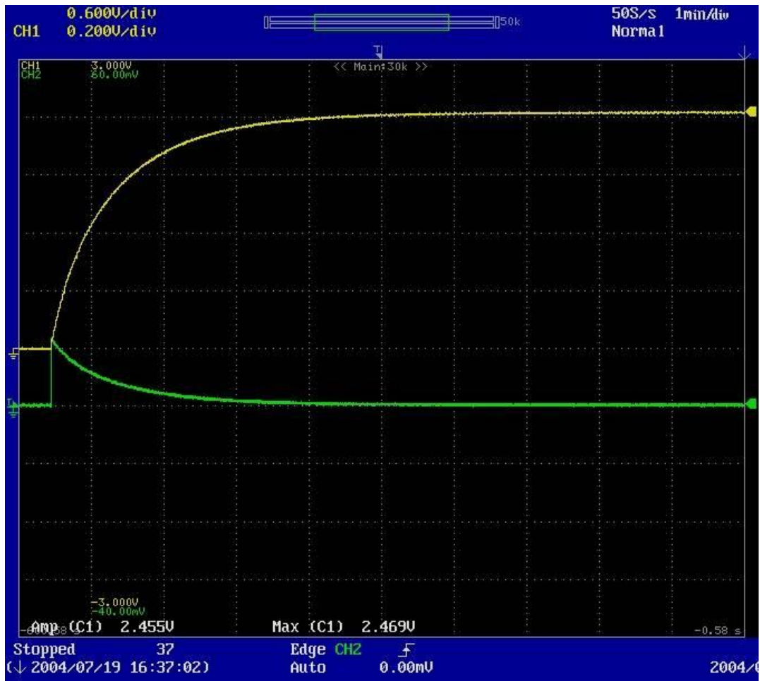
Figure A1.1-13: Oscilloscope Screen Capture of 25 A Charge Cycle at T=50°C (Timescale: 1 min/div)
