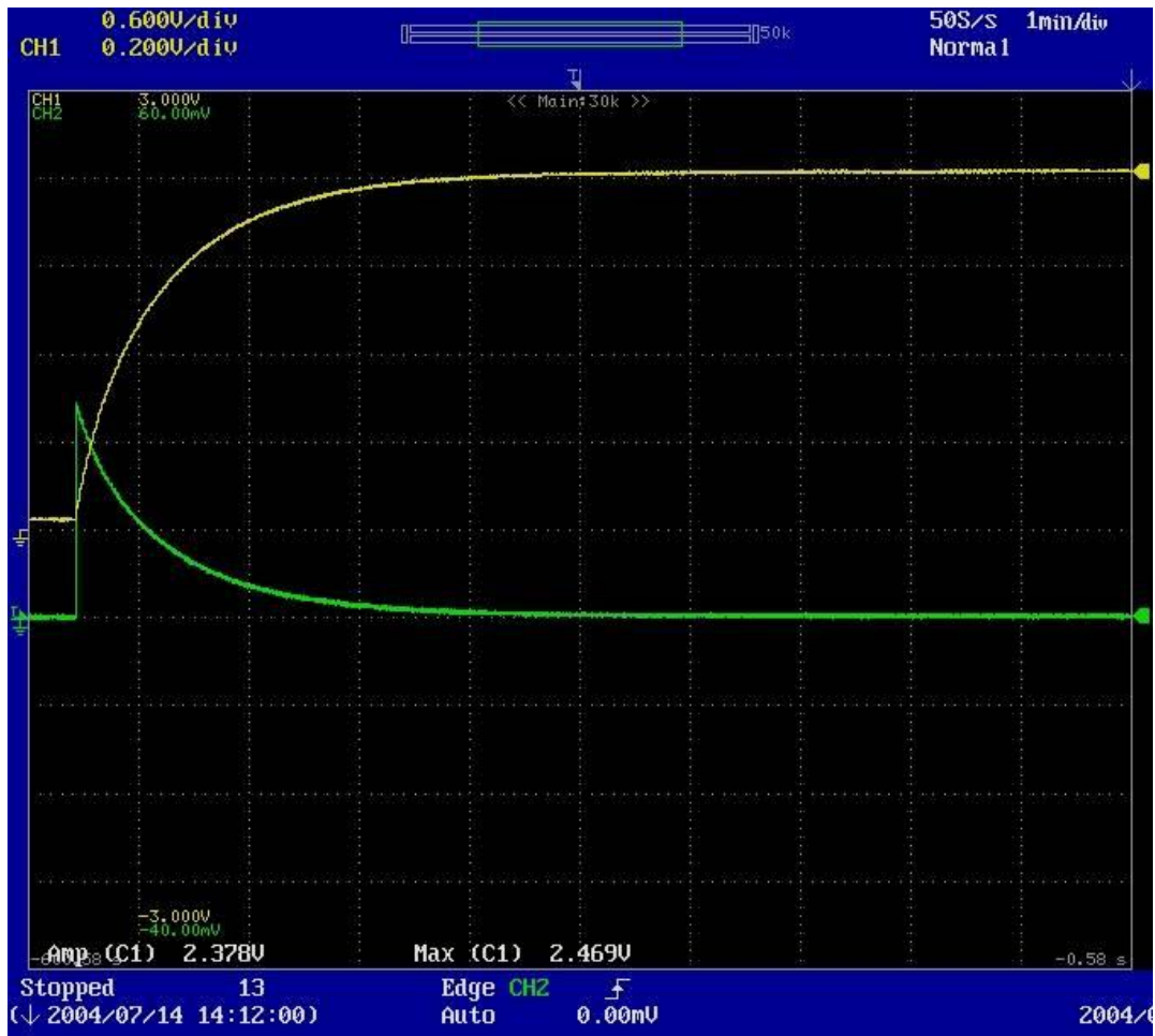
Figure A2.3-13: Oscilloscope Screen Capture of 60 A Charge Cycle at T=50^{\circ}\text{C} (Timescale: 1 min/div)
