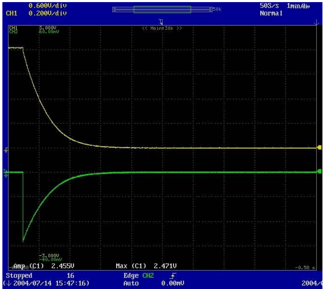
Figure A2.3-7: Oscilloscope Screen Capture of 60 A Discharge Cycle at T = 0^{\circ}\text{C} (Timescale: 1 min/div)
