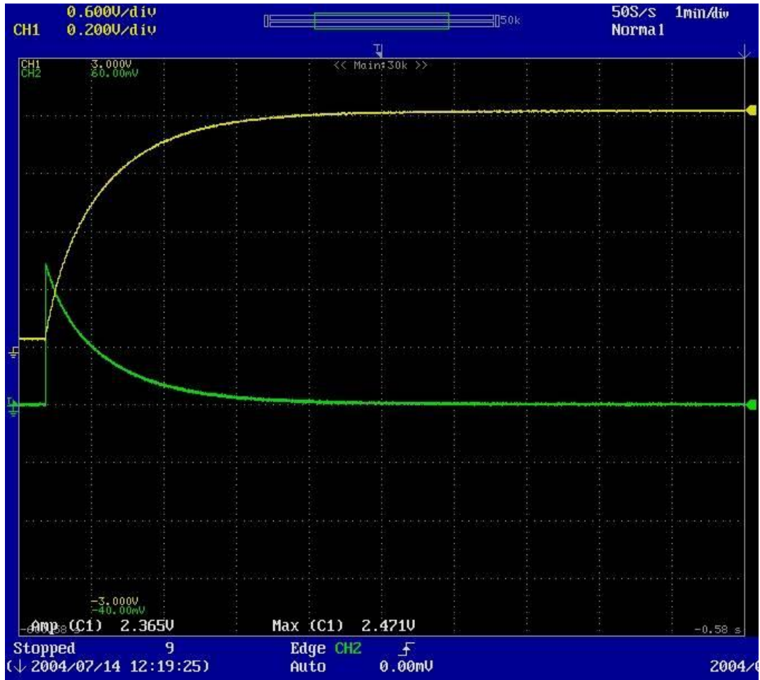
Figure A2.3-9: Oscilloscope Screen Capture of 60 A Charge Cycle at T = 25^{\circ}\text{C} (Timescale: 1 min/div)
