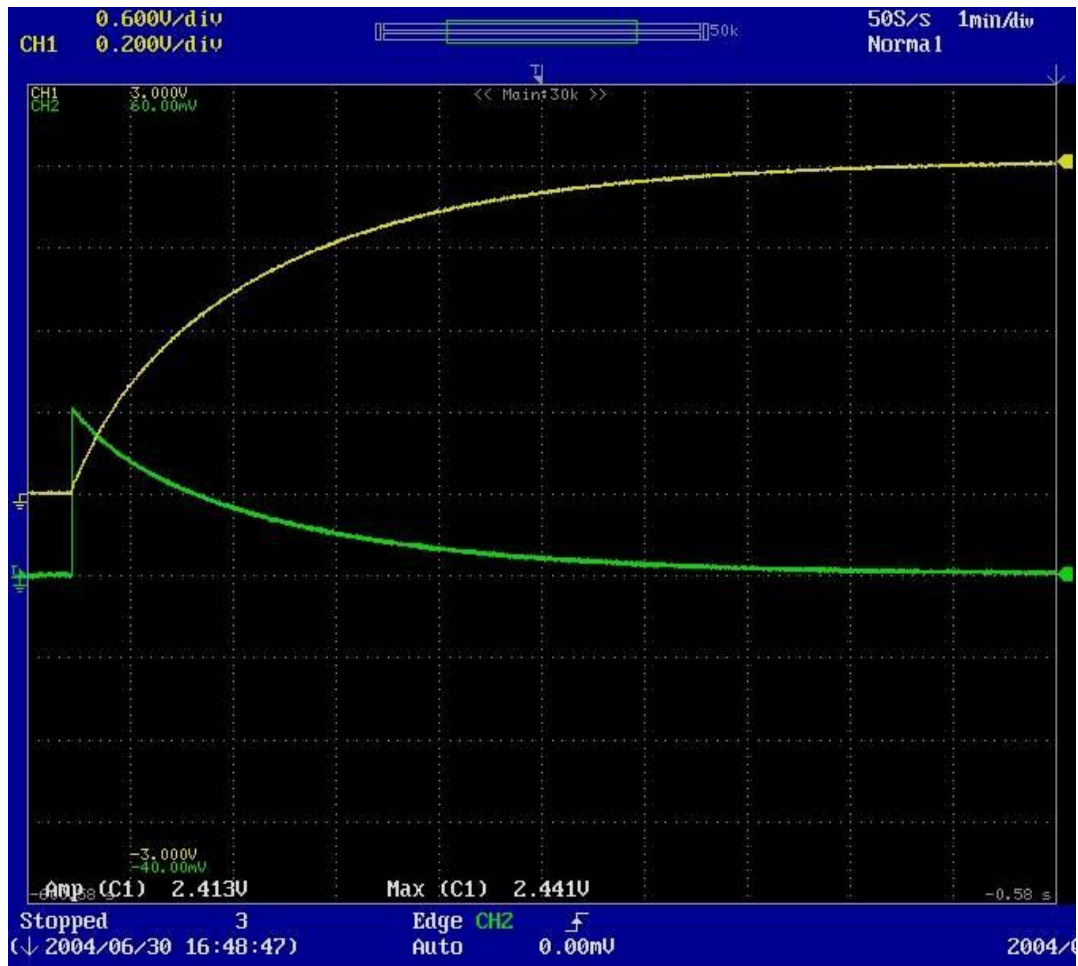
Figure A3.2-5: Oscilloscope Screen Capture of 50 A Charge Cycle at T=0^{\circ}\text{C} (Timescale: 1 min/div)
