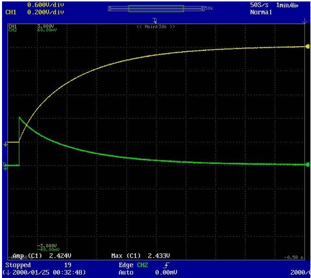
Figure A3.2-9: Oscilloscope Screen Capture of 50 A Charge Cycle at T = 25^{\circ}\text{C} (Timescale: 1 min/div)
