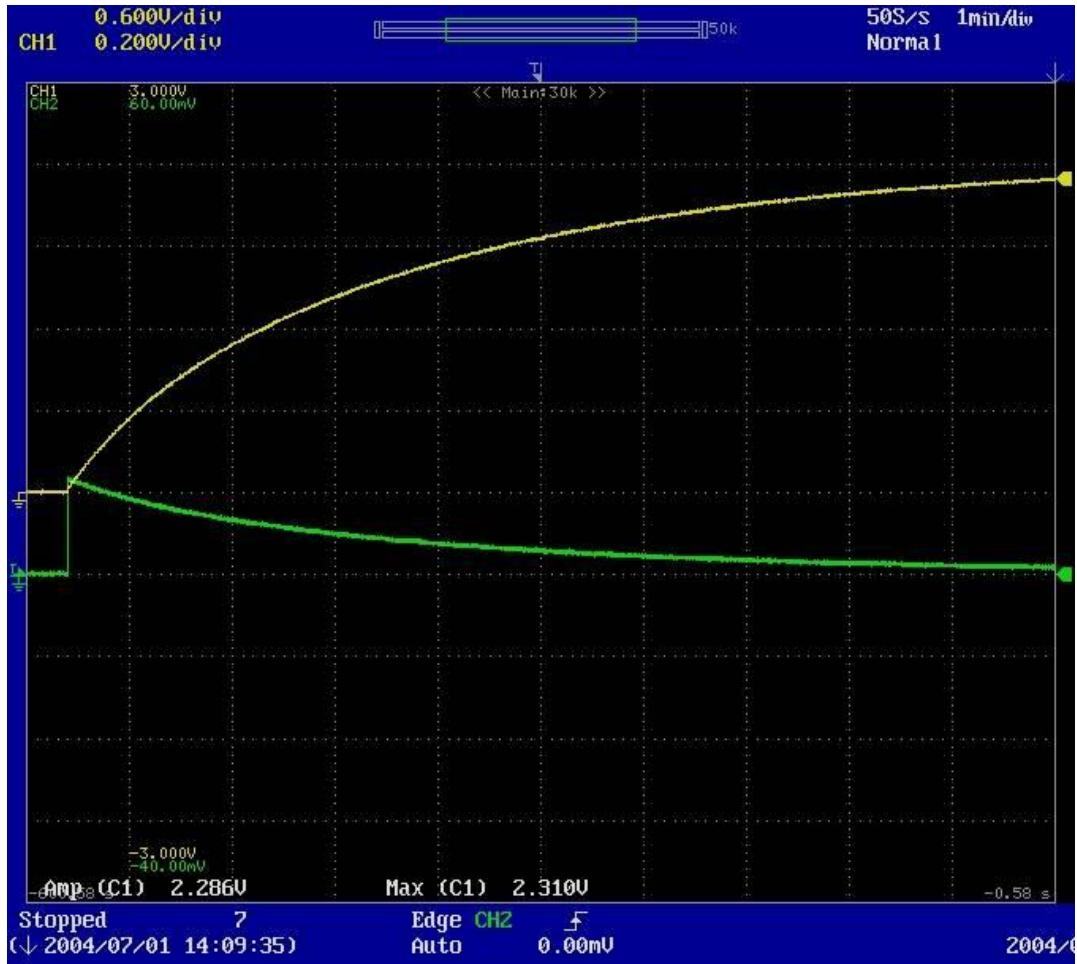
Figure A3.1-1: Oscilloscope Screen Capture of 25 A Charge Cycle at T = -25^{\circ}\text{C} (Timescale: 1 min/div)
