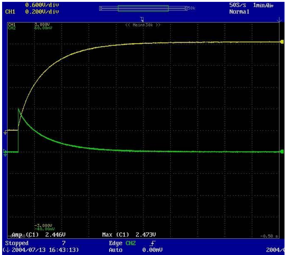
Figure A2.2-1: Oscilloscope Screen Capture of 50 A Charge Cycle at T = -25^{\circ}\text{C} (Timescale: 1 min/div)
