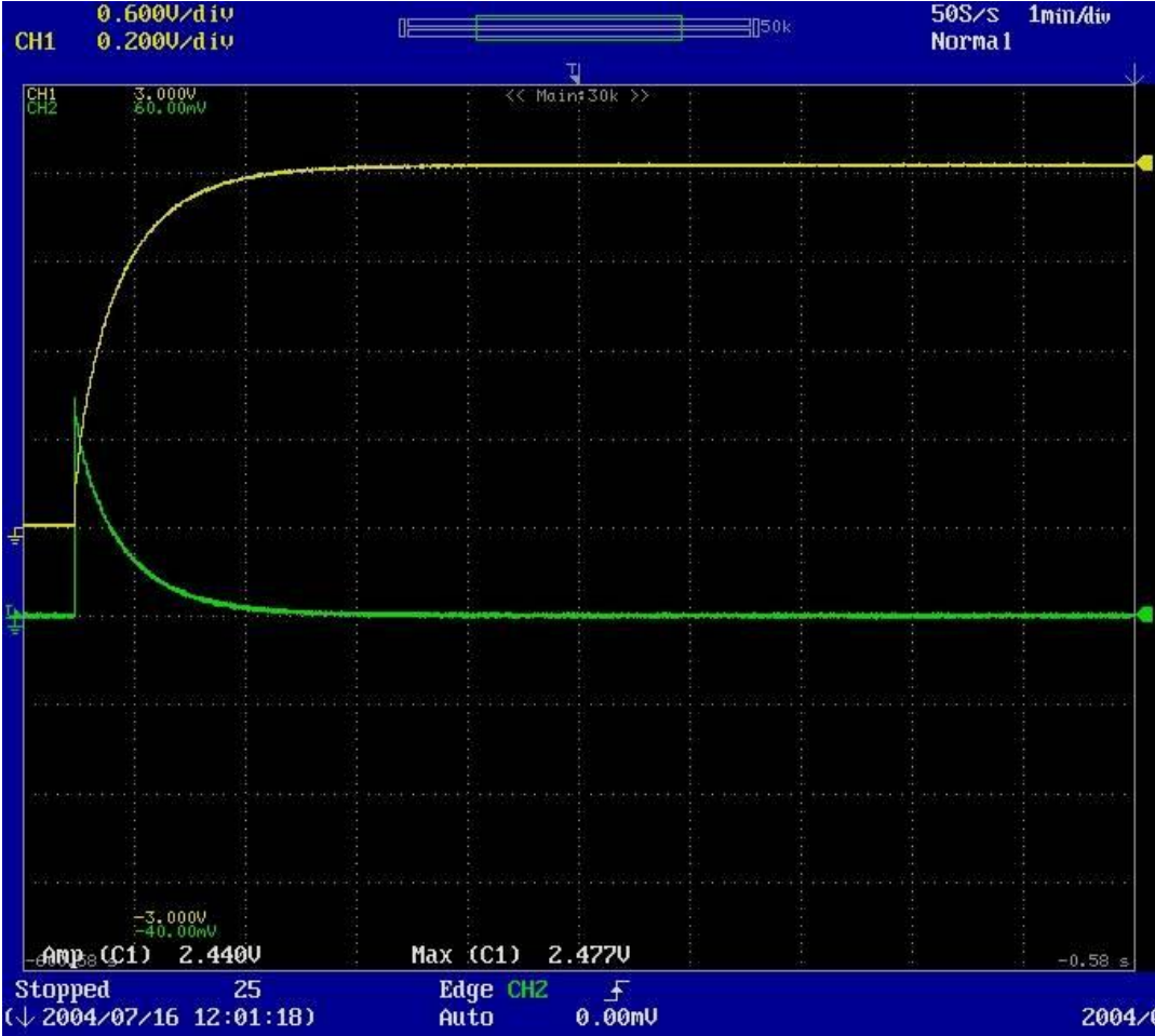
Figure A1.3-1 Oscilloscope Screen Capture of 60 A Charge Cycle at T= -25°C (Timescale: 1 min/div)
