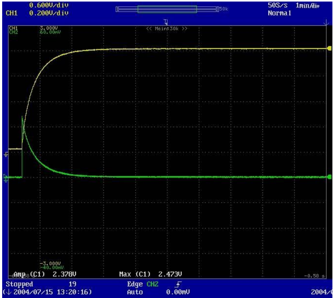
Figure A1.3-9: Oscilloscope Screen Capture of 60 A Charge Cycle at T = 25^{\circ}\text{C} (Timescale: 1 min/div)
