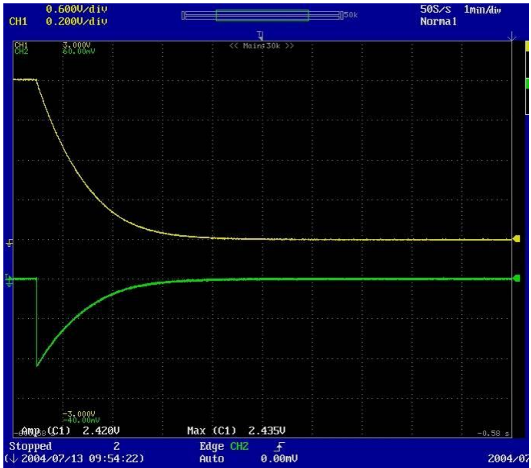
Figure A2.2-11: Oscilloscope Screen Capture of 50 A Discharge Cycle at T=25°C (Timescale: 1 min/div)
