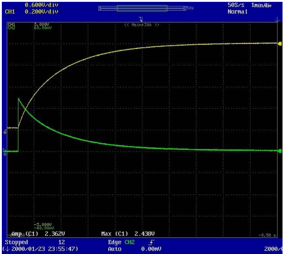
Figure A3.3-13: Oscilloscope Screen Capture of 60 A Charge Cycle at T = 50^{\circ}\text{C} (Timescale: 1 min/div)
