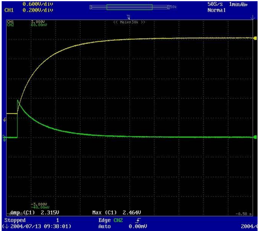
Figure A2.2-9: Oscilloscope Screen Capture of 50 A Charge Cycle at T= 25°C (Timescale: 1 min/div)
