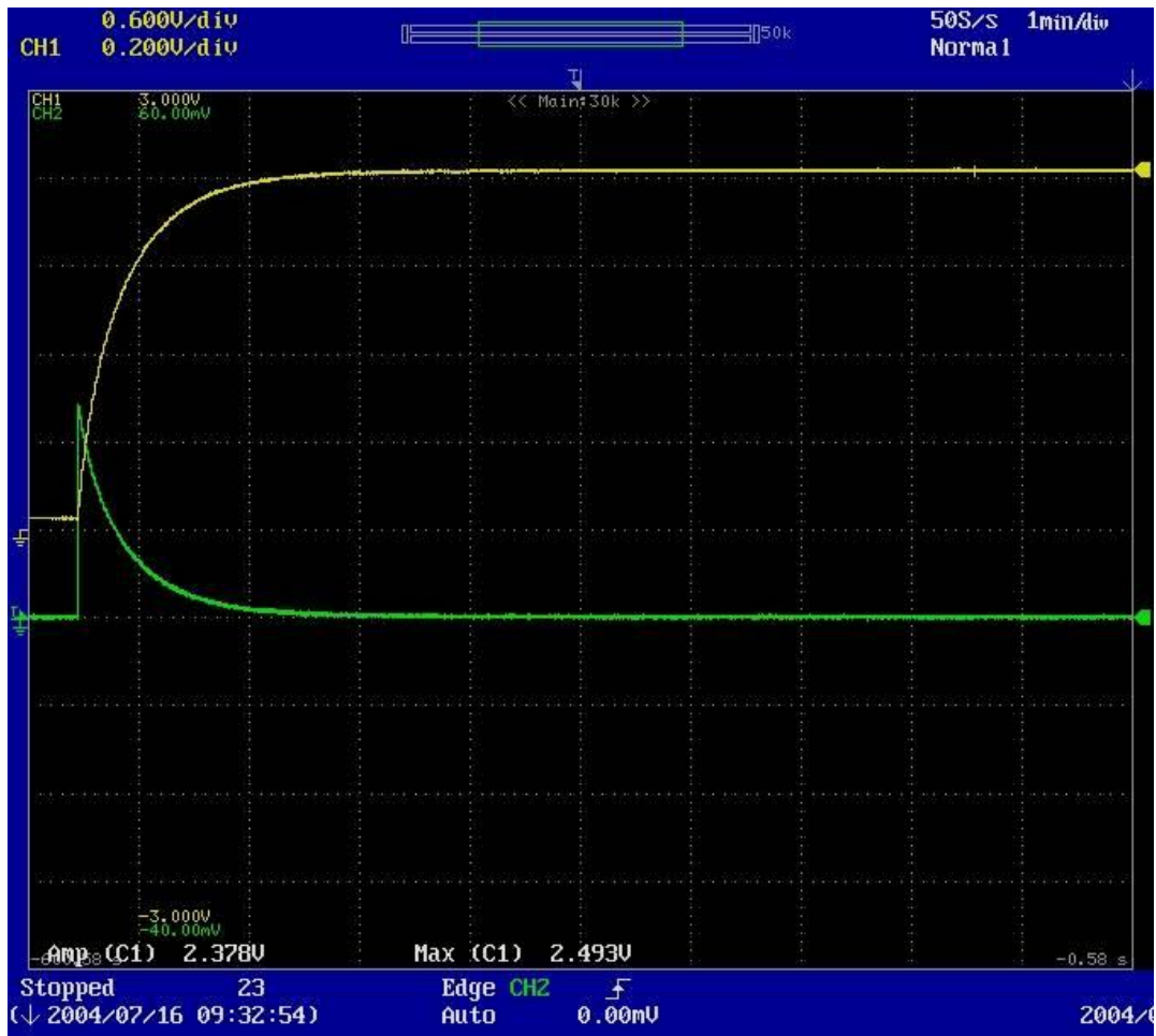
Figure A1.3-5: Oscilloscope Screen Capture of 60 A Charge Cycle at T=0^{\circ}\text{C} (Timescale: 1 min/div)
