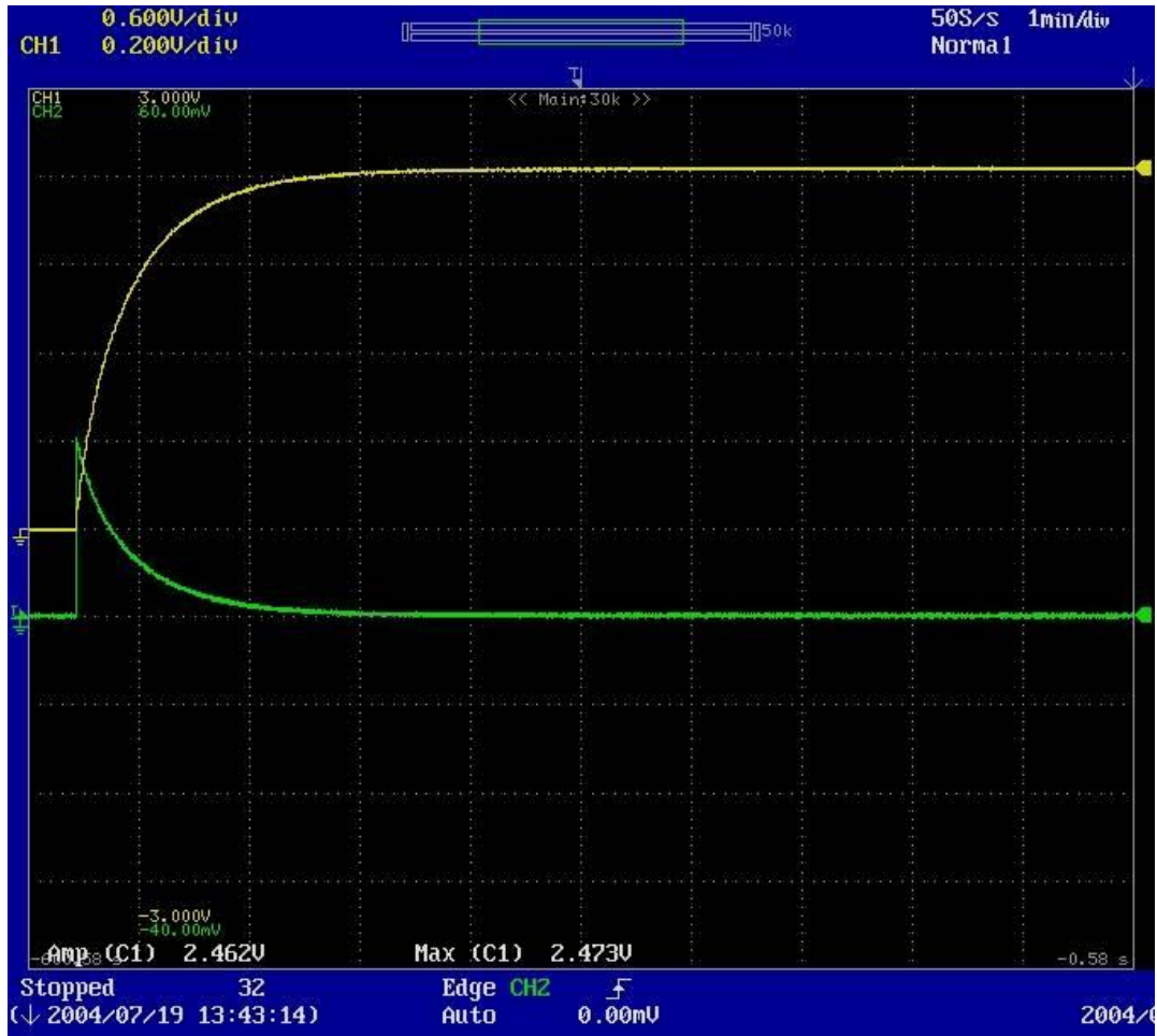
Figure A1.2-9: Oscilloscope Screen Capture of 50 A Charge Cycle at T = 25^{\circ}\text{C} (Timescale: 1 min/div)
