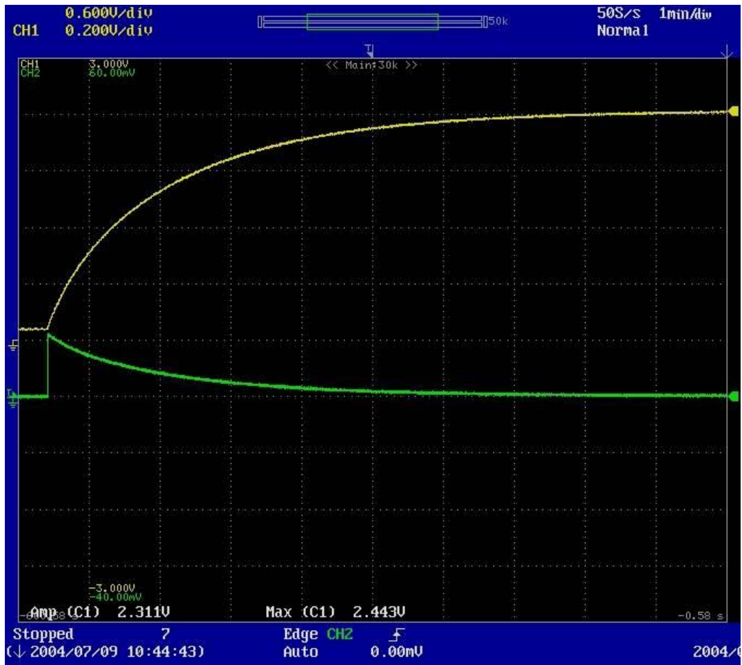
Figure A2.1-5: Oscilloscope Screen Capture of 25 A Charge Cycle at T = 0^{\circ}\text{C} (Timescale: 1 min/div)
