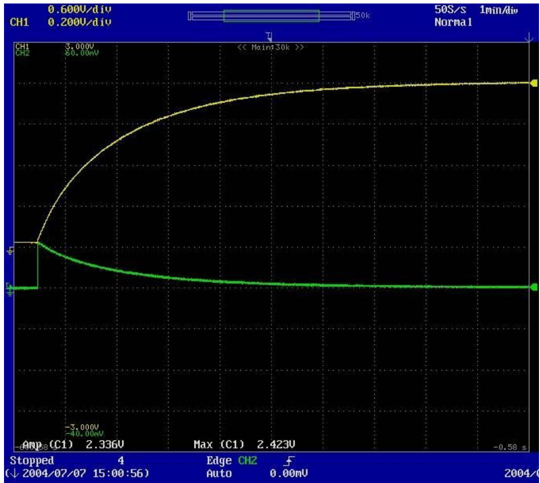
Figure A2.1-13: Oscilloscope Screen Capture of 25 A Charge Cycle at T = 50^{\circ}\text{C} (Timescale: 1 min/div)
