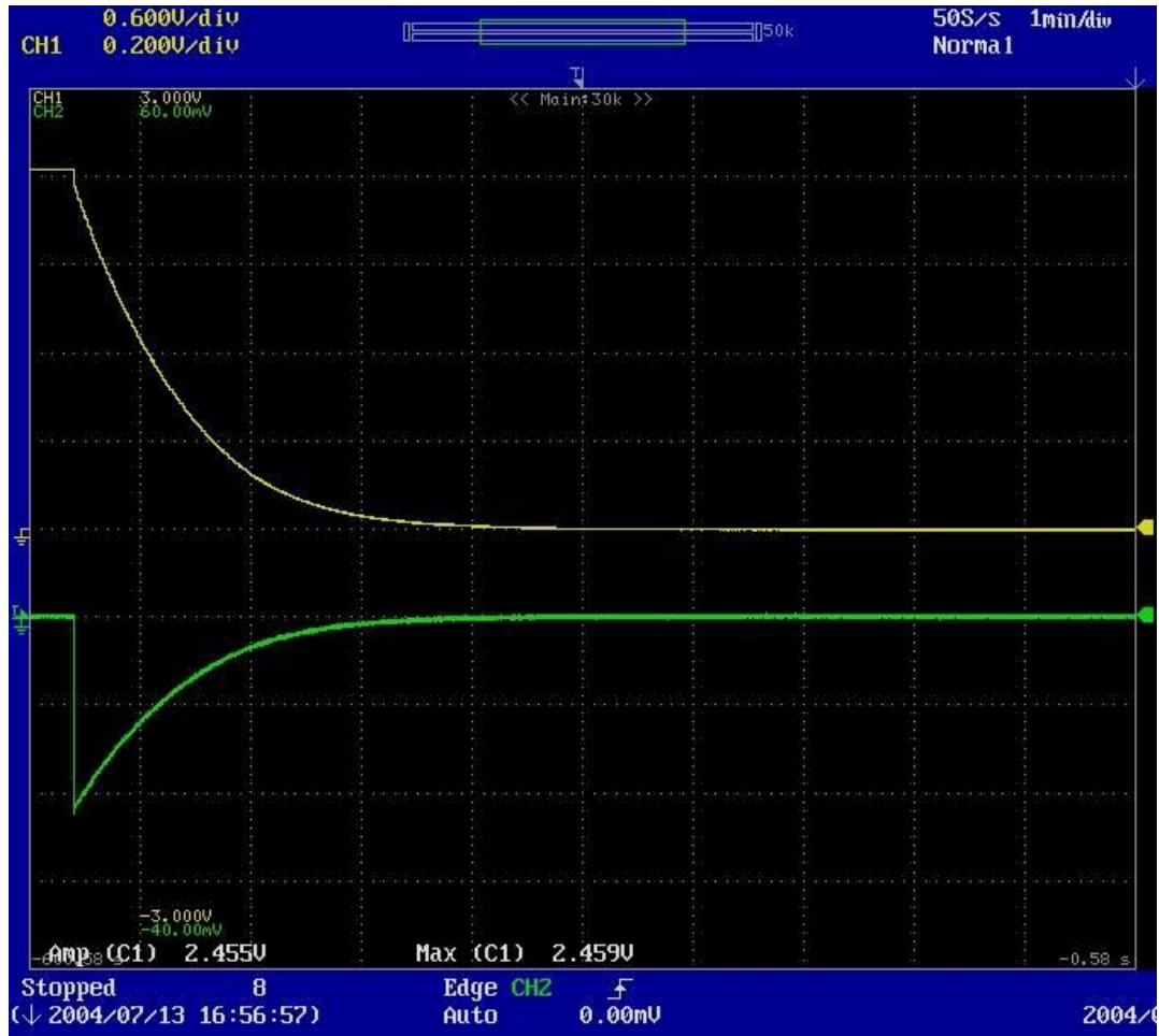
Figure A2.2-3: Oscilloscope Screen Capture of 50 A Discharge Cycle at T = -25^{\circ}\text{C} (Timescale: 1 min/div)
