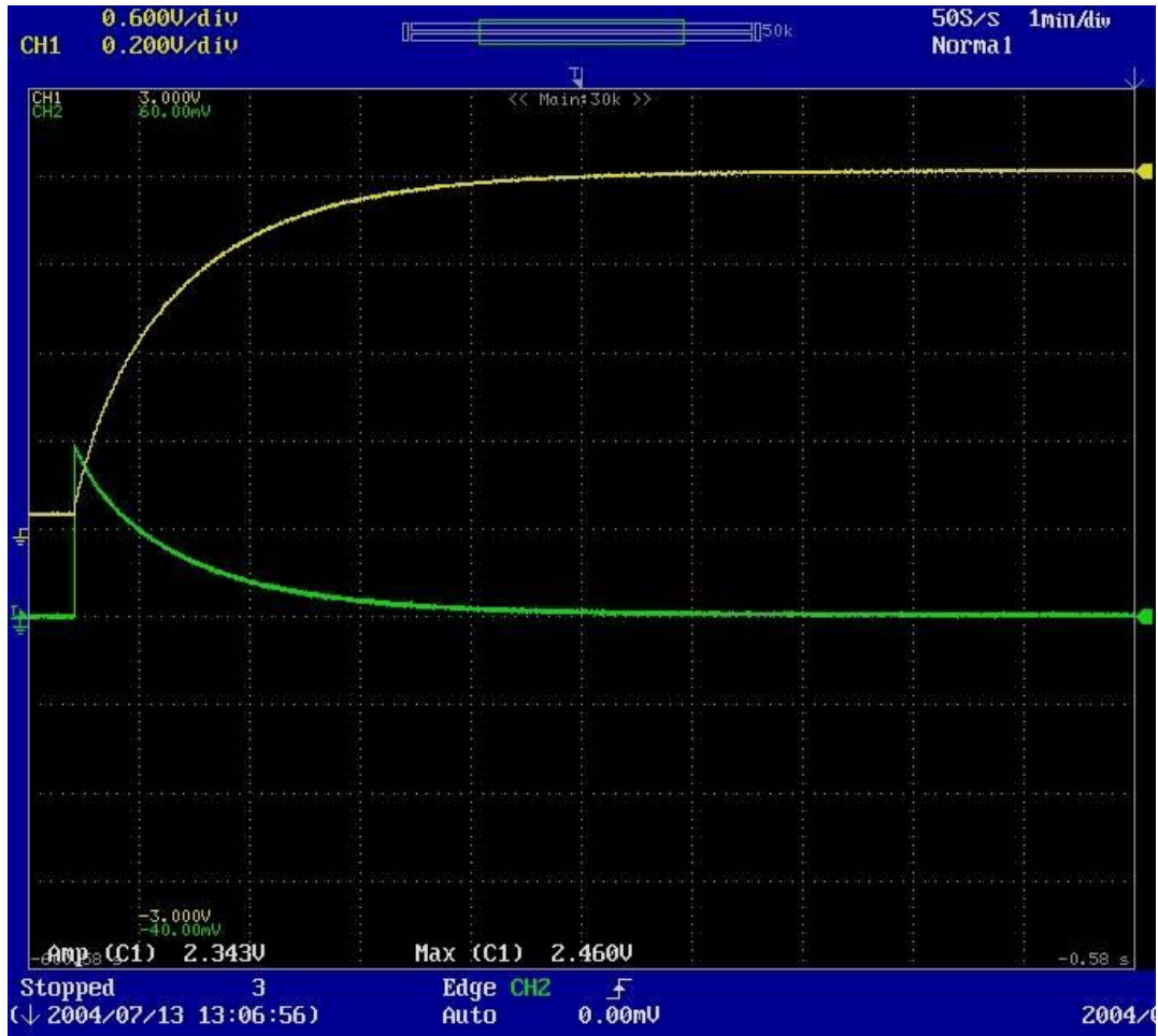
Figure A2.2-13: Oscilloscope Screen Capture of 50 A Charge Cycle at T = 50^{\circ}\text{C} (Timescale: 1 min/div)
