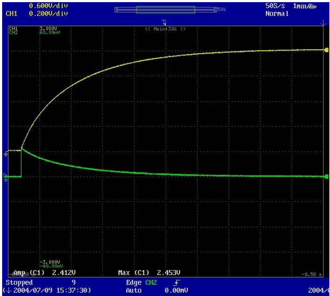
Figure A2.1-1: Oscilloscope Screen Capture of 25 A Charge Cycle at T = -25^{\circ}\text{C} (Timescale: 1 min/div)
