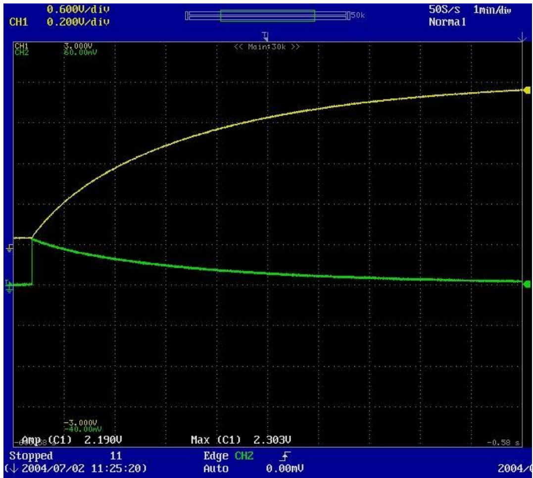
Figure A3.1-9: Oscilloscope Screen Capture of 25 A Charge Cycle at T = 25^{\circ}\text{C} (Timescale: 1 min/div)
