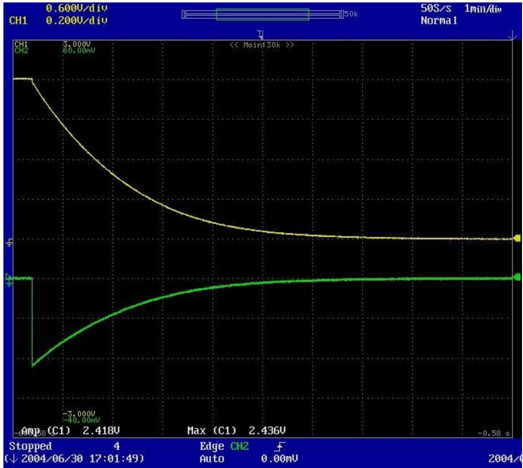
Figure A3.2-7: Oscilloscope Screen Capture of 50 A Discharge Cycle at T=0^{\circ}\text{C} (Timescale: 1 min/div)
