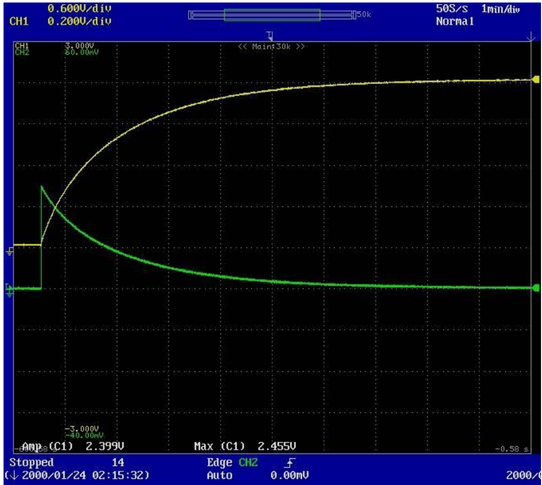
Figure A3.3-5: Oscilloscope Screen Capture of 60 A Charge Cycle at T = 0^{\circ}\text{C} (Timescale: 1 min/div)
