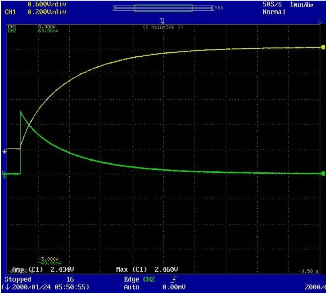
Figure A3.3-1: Oscilloscope Screen Capture of 60 A Charge Cycle at T= -25°C (Timescale: 1 min/div)
