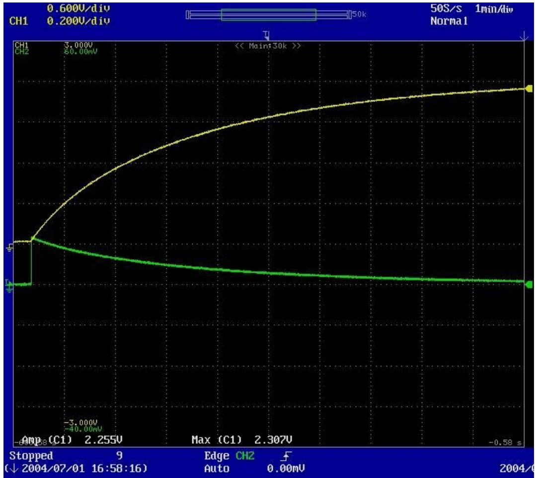
Figure A3.1-5: Oscilloscope Screen Capture of 25 A Charge Cycle at T = 0^{\circ}\text{C} (Timescale: 1 min/div)
