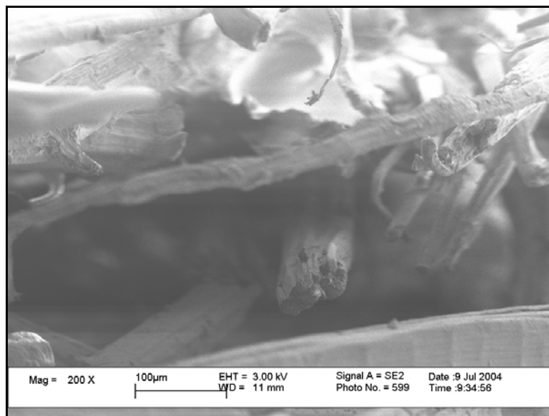
Figure 49 SEM Photo of Kenaf PVAc composite cross-section. At Magnification 400X
