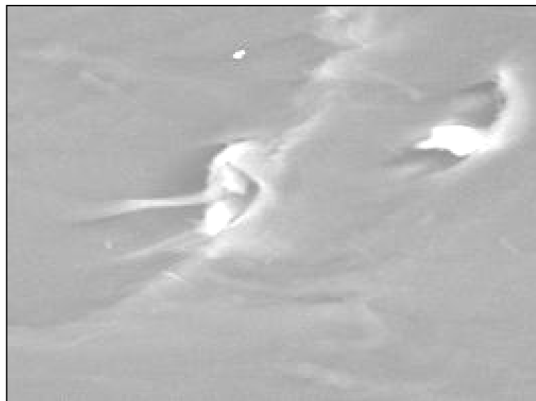
Figure 34 SEM Pictures of Cotton-Flax-Eastar Composites. (Exhibiting Good Bonding)
