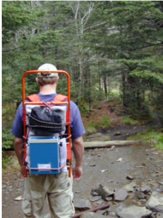
Figure 3.1. Portable Ozone Monitor in Canopy
