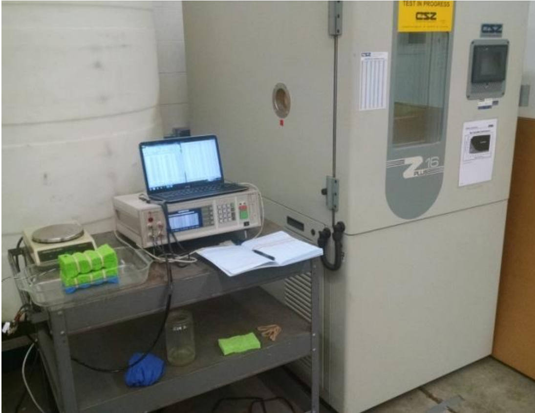
Figure 7: Photograph of the environmental testing chamber and LRC meter setup for data gathering.
