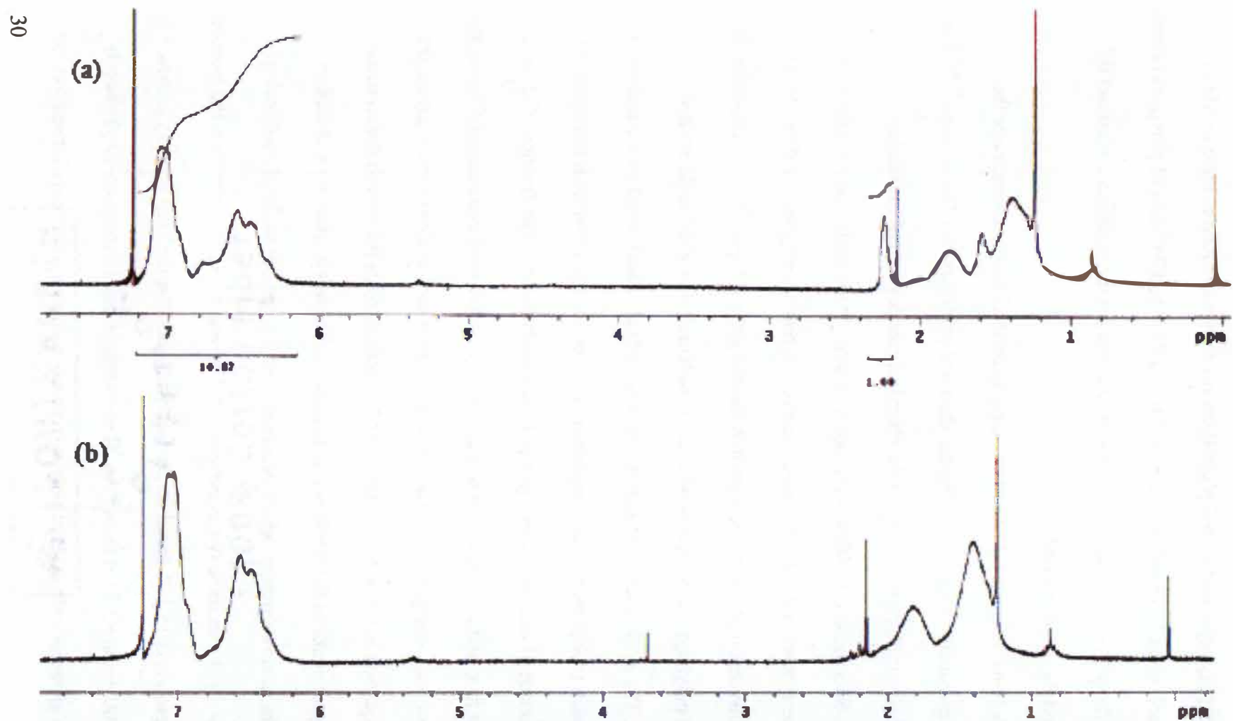
Figure 2.3 ^1\text{H} spectra of (a) poly(styrene-co-acetoxystyrene) copolymers and (b) poly(styrene-co-vinyl phenol) copolymers after hydrolysis.
