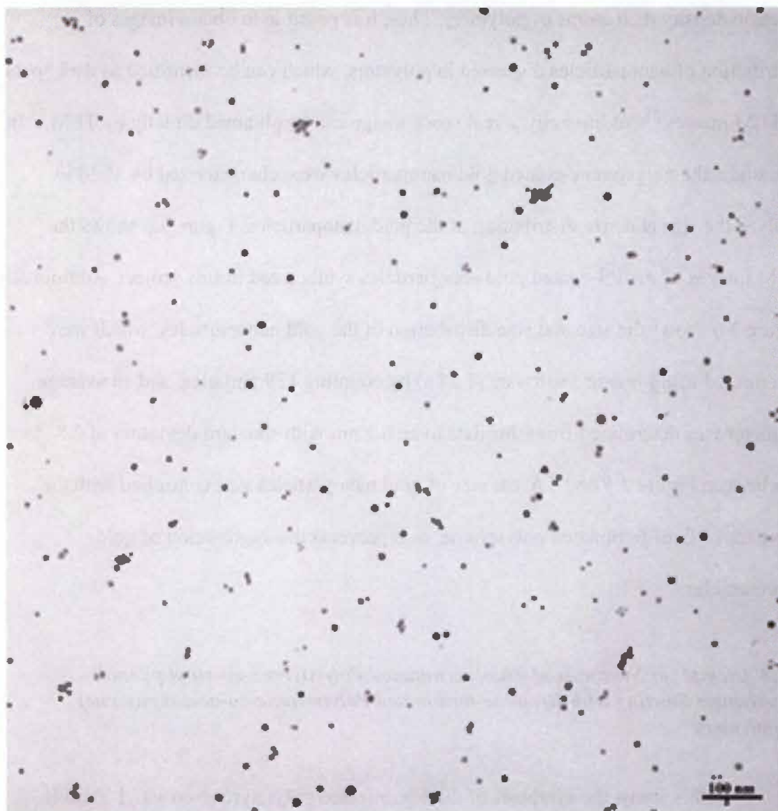
Figure 3.5 Representative TEM image of PS-coated gold nanoparticles. (Scale bar size: 100 nm)
