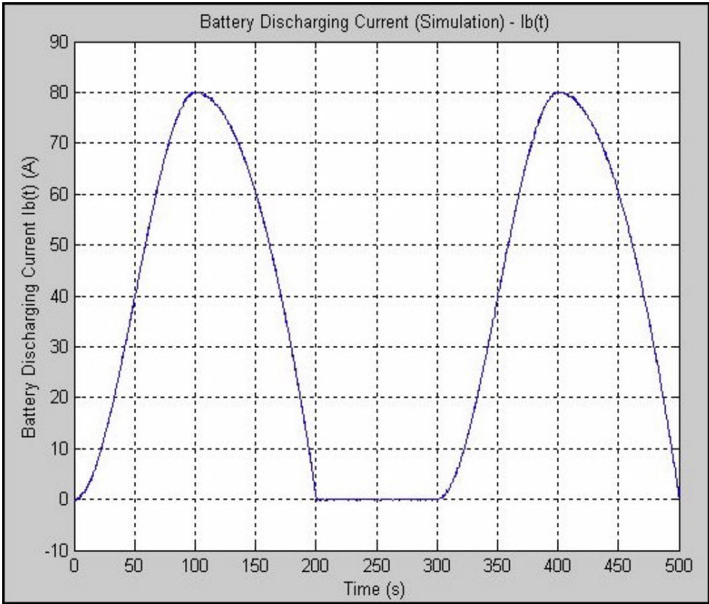
Figure 9. Battery discharging current I_b(t) used in simulation
