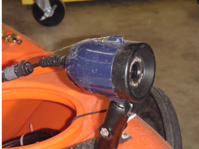
Figure 212: A photo of the Deep Blue waterproof digital camera mounted on top of the kayak.
