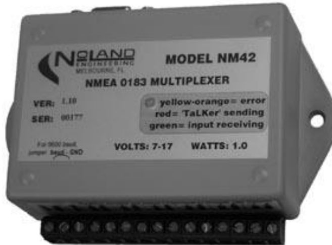
Figure 20: A picture of a NMEA 0183 multiplexer used to combine depth data and GPS data into a single data string.
