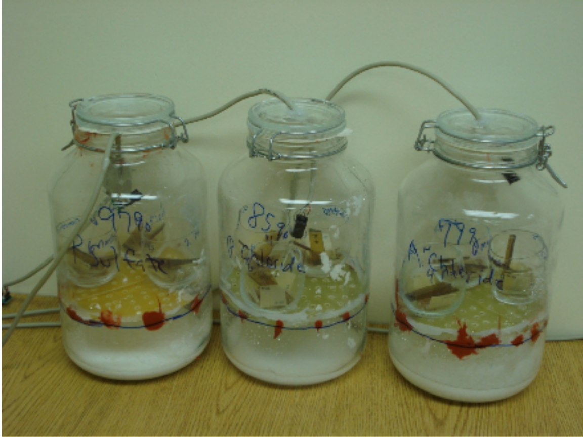
Figure A.1 Constant relative humidity aging in sealed jars
