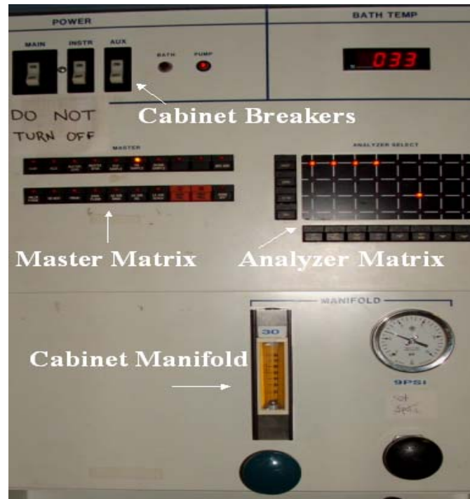
Figure 3.12. Control Panel of the Horiba Instrument Cabinet.
