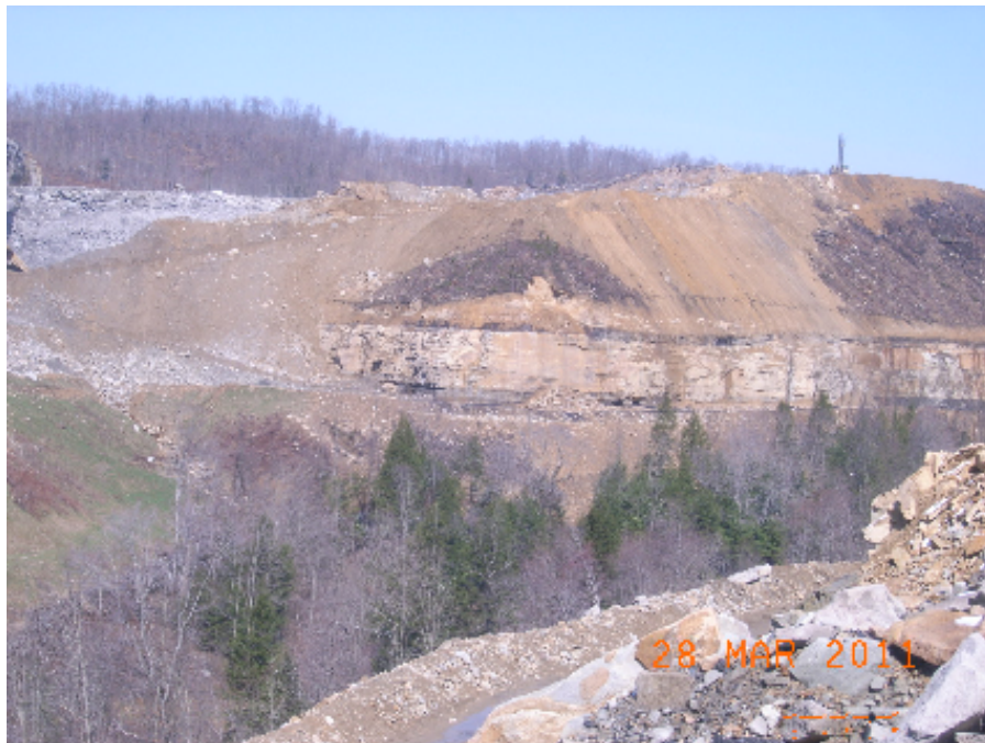
Figure 25: Site Photo A - Grey highwall above that is a cut-through the ridge. This ridge was added after the original permit was issued (Curry).
