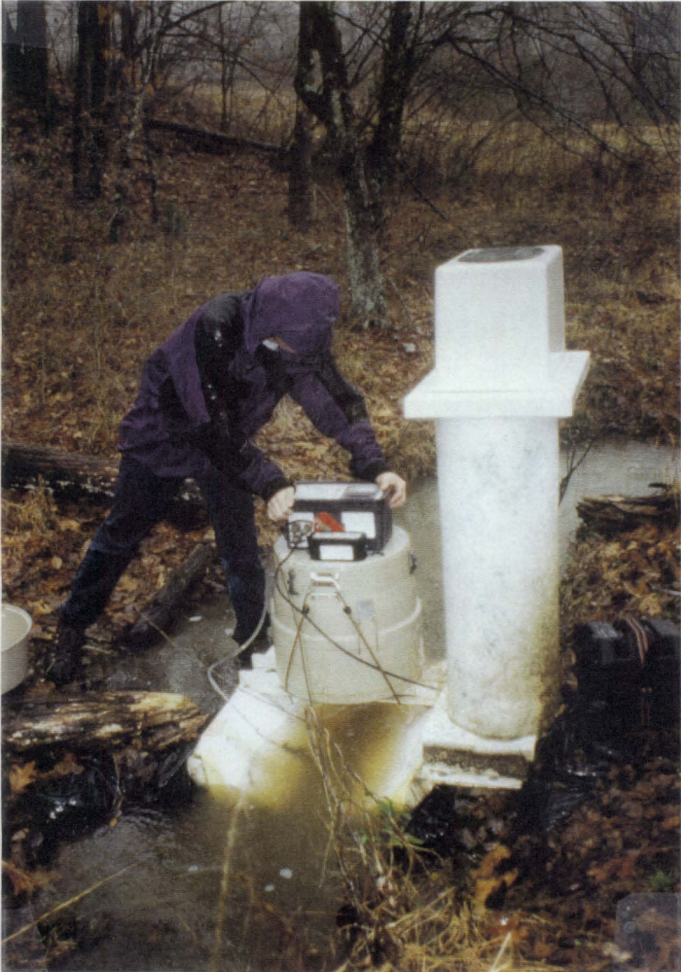
Figure 11. Trapezoidal flume equipped with Stevens recorder and autosampler.
