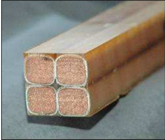
Figure 4.10 Photograph of a 2x2 Conductor Assembly [8]. Conductors are impregnated with and held together by CTD-403 resin.
