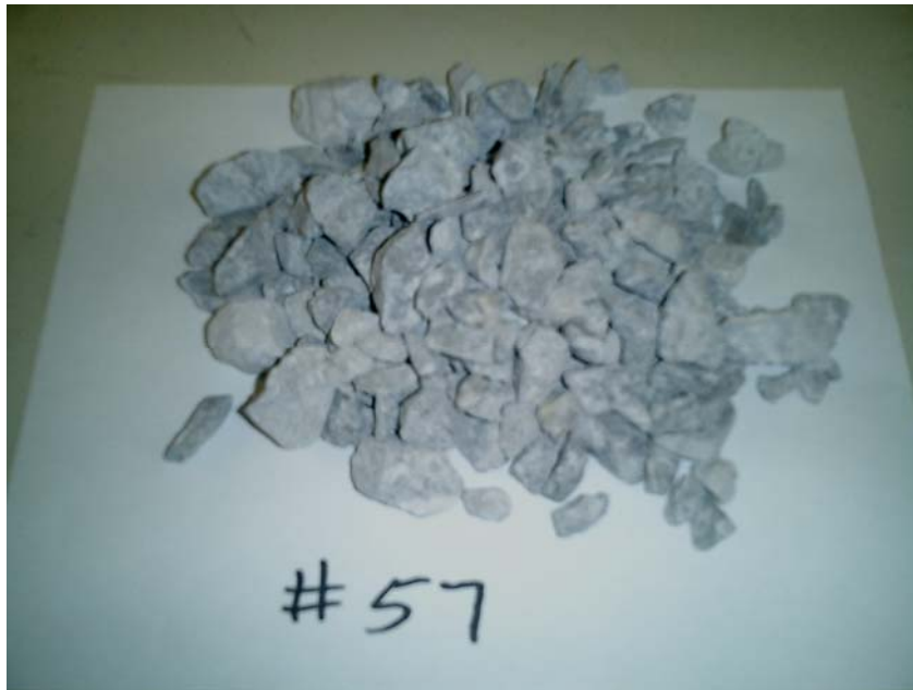
Figure B-2 #57 Coarse Aggregate
