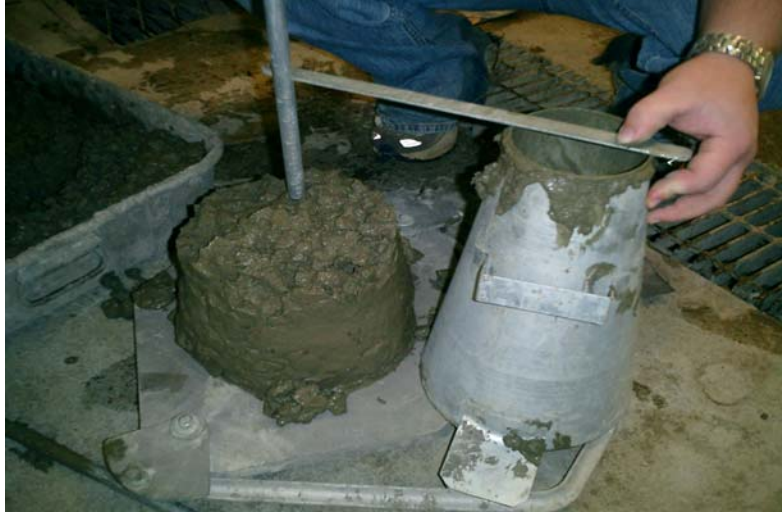
Figure B-8 Slump Test in Progress
