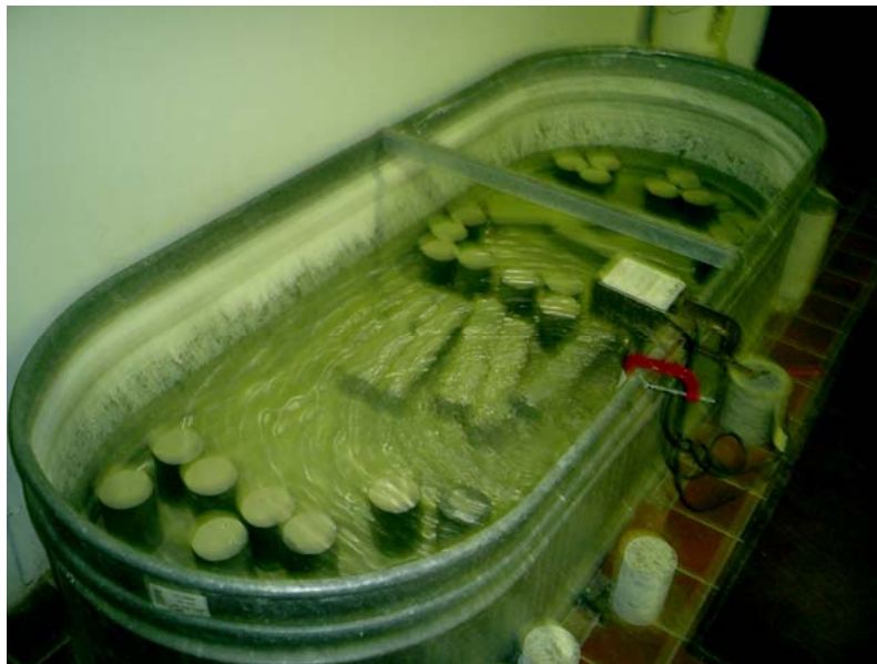
Figure B-7 Lime Water Bath
