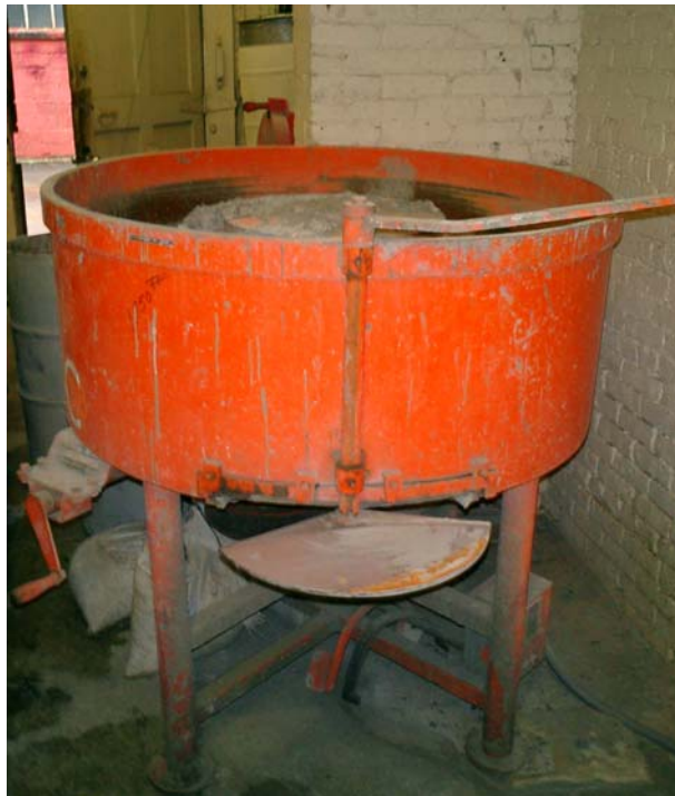
Figure B-5 Laboratory Mixer (7.5 ft 3 capacity)
