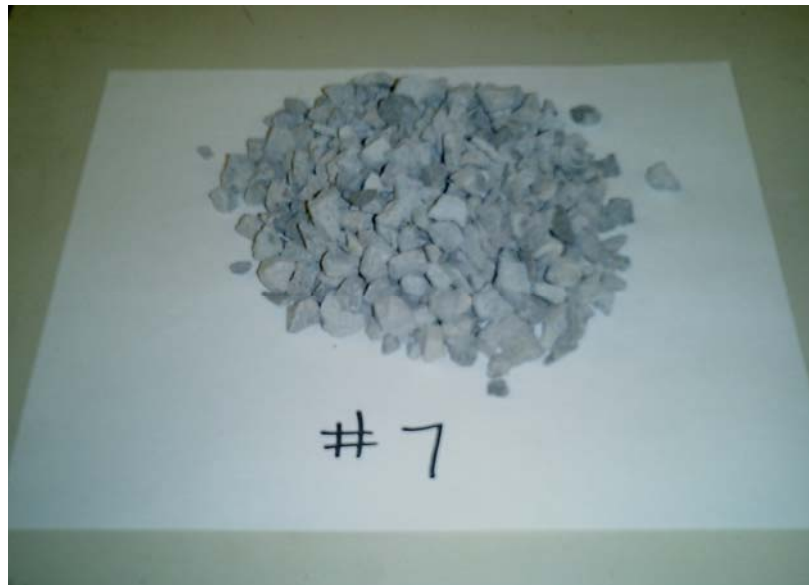
Figure B-3 #7 Coarse Aggregate
