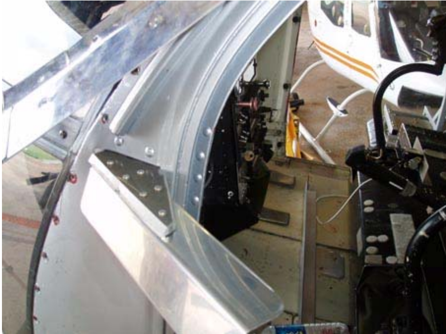
Figure 47. Upper Hinge Brace (Installed).
