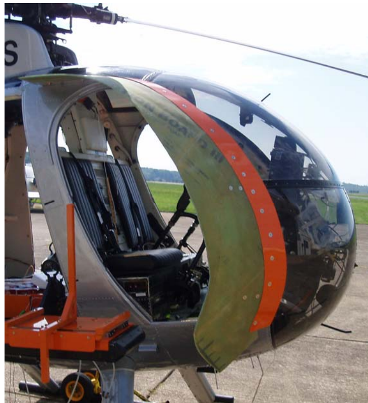
Figure 52. Deflector Installed on Right Side...
