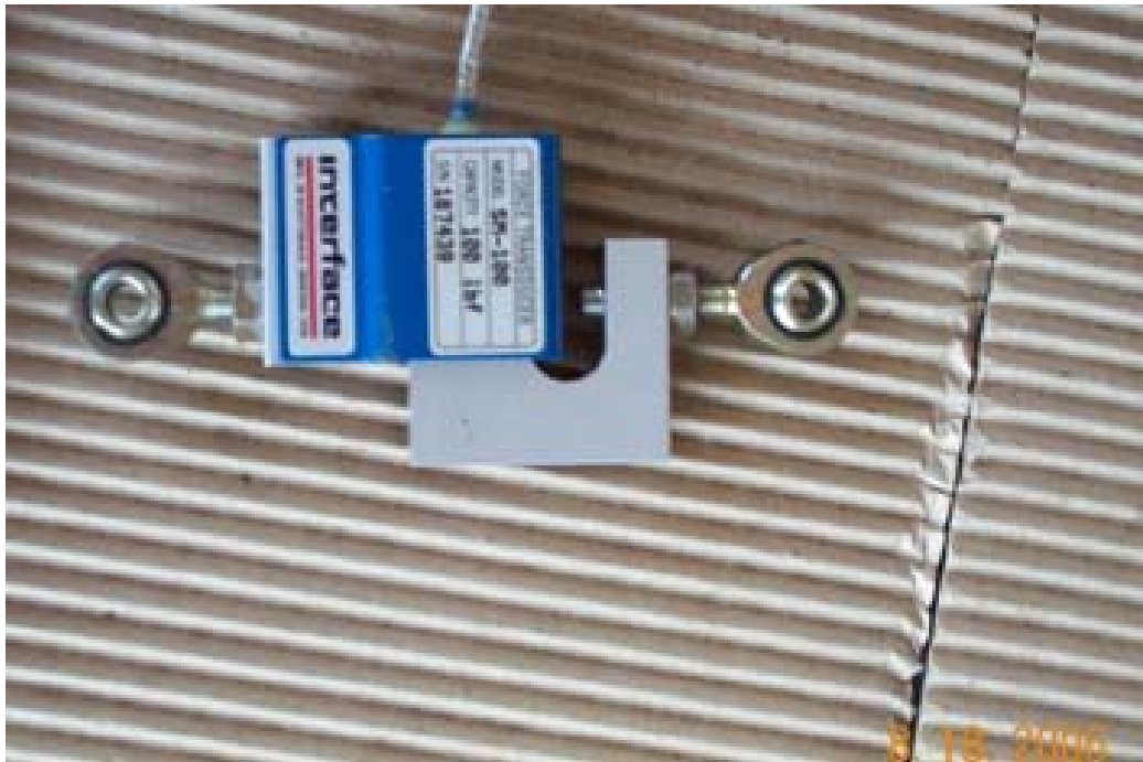
Figure 61. Manikin Longitudinal Force Load Cell.
