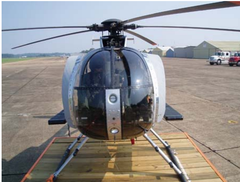
Figure 67. 40 Degree 12 Inch Deflector (Installed).
