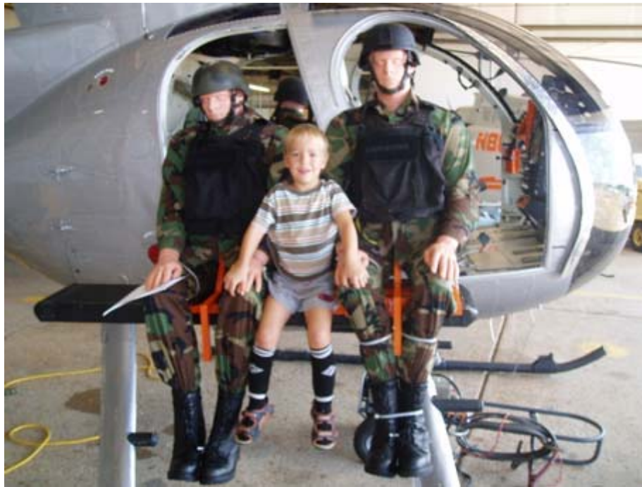
Figure 65. External Passenger Bench with Manikins Installed.
