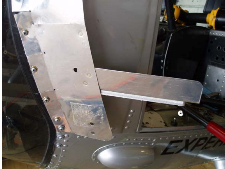
Figure 17. Left Lower Hinge Brace Installation.
