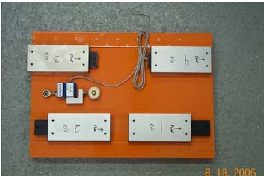
Figure 62. Manikin Roller Seat Assembly with Load Cell Location.
