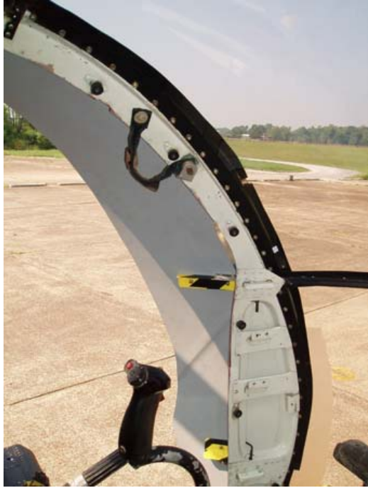
Figure 53. Pilot Field-of-View with 40 Degree 12 Inch Deflector Installed (Left)
