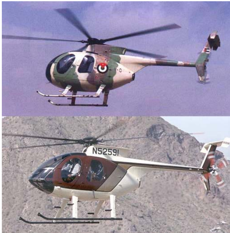
Figure 6. Comparison of round- and pointed-nose MD-500 variants.
