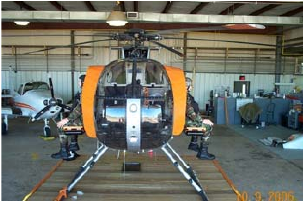
Figure 68. 40 Degree 10 Inch Deflector (Installed).
