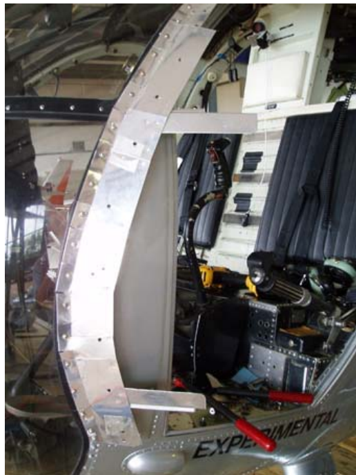
Figure 48. Leading Edge Metal Fixture with Hinge Braces (Installed, Complete).
