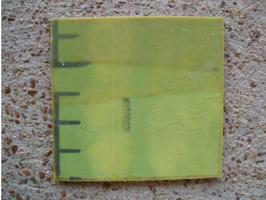
Figure 55. Deflector Material Test Section (Bending).
