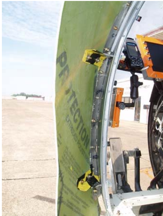
Figure 50. Deflector Attached to Full Leading Edge Fixture
