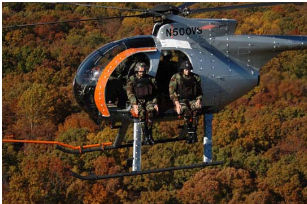
Figure 39. Test Aircraft in Flight with 50° 8-inch deflector with Gurney Flap.
