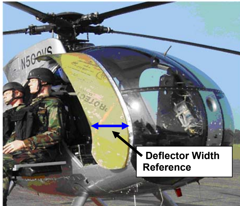
Figure 16. Prototype Deflector Mounted on MD-500 with Simulated EP.
