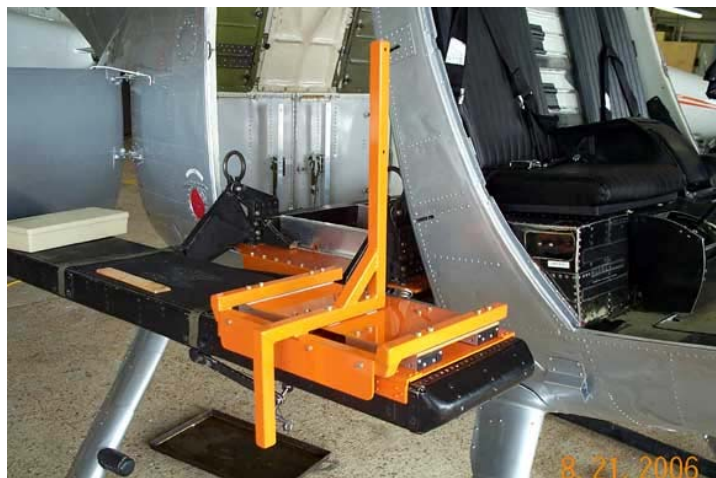
Figure 26. External Passenger Bench with Manikin Instrumentation.
