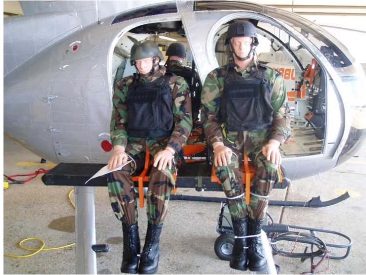
Figure 27. External Passenger Manikins on Bench.
