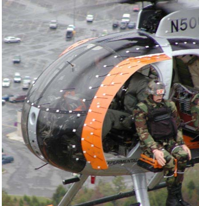
Figure 77. 50 Degree 8 Inch in-flight Flow Visualization (Left Close-Up).
