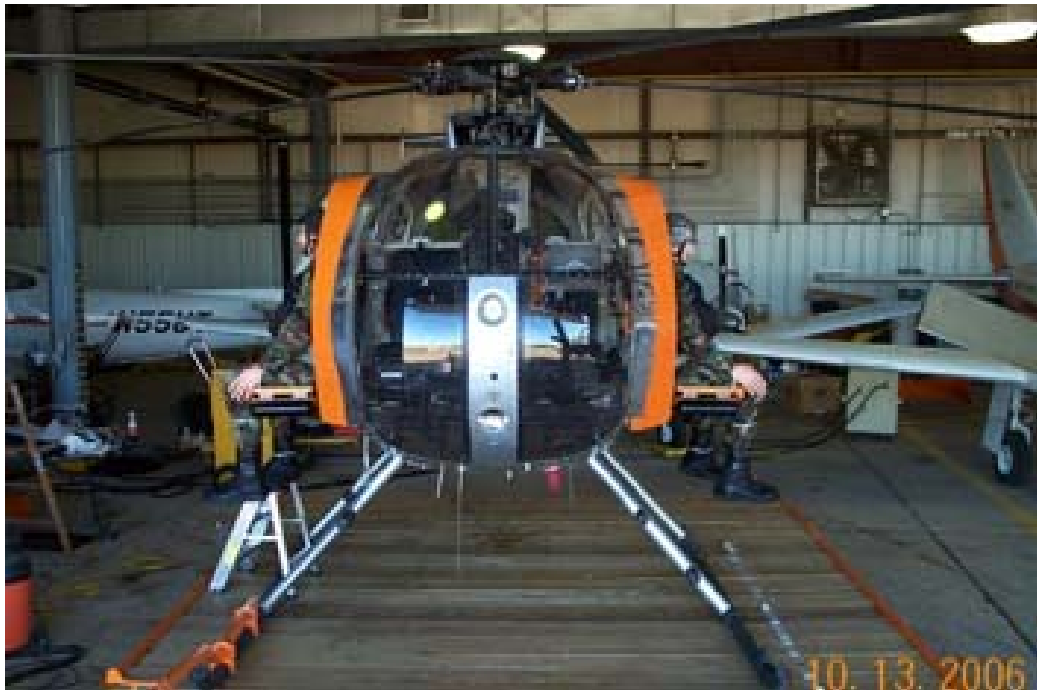
Figure 70. 50 Degree 10 Inch Deflector (Installed).
