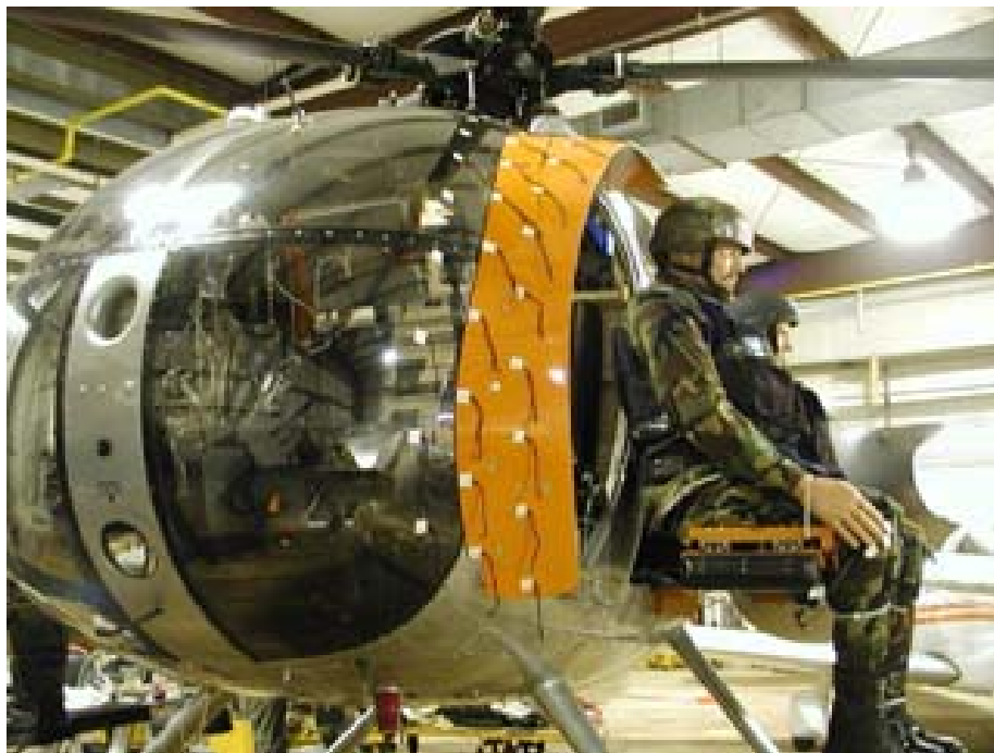
Figure 72. 50 Degree 8 Inch Deflector with Flow Visualization Tufts.
