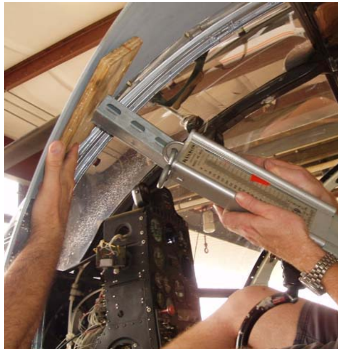
Figure 59. Static Load Testing of Installed Deflector (1).
