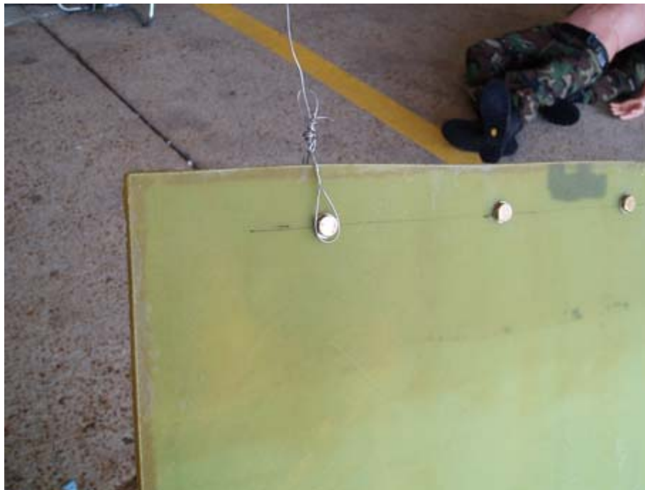
Figure 58. Deflector Test Section Tear Out Test.
