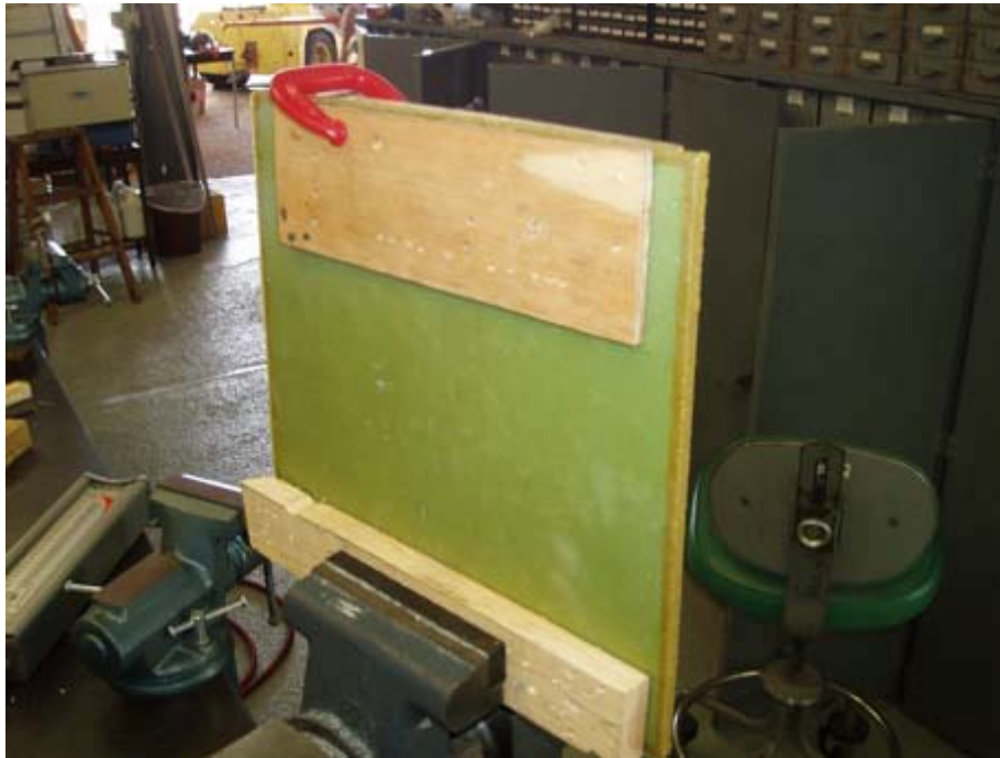
Figure 56. Deflector Test Section Bending Test.
