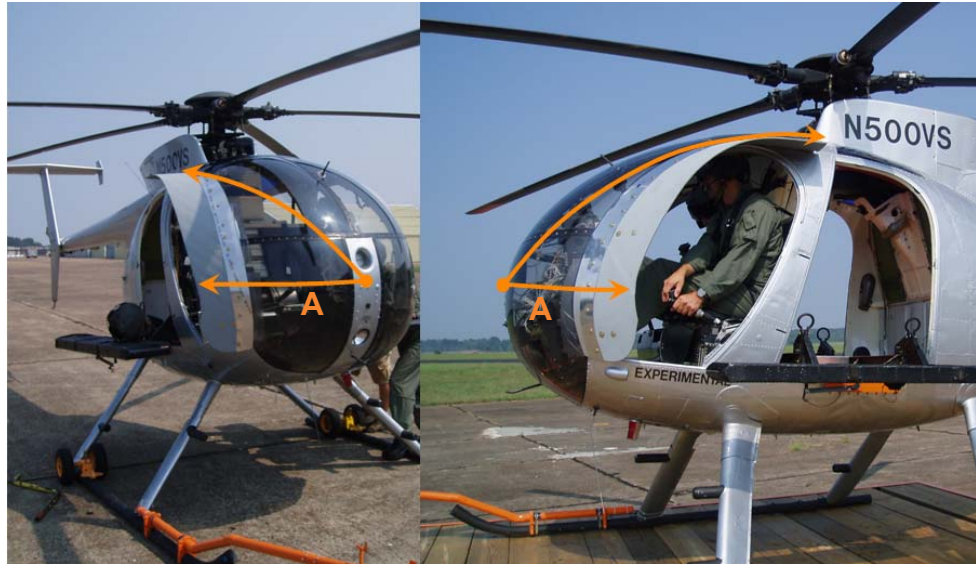
Figure 21. Measurement of Deflector Characteristic Length.
