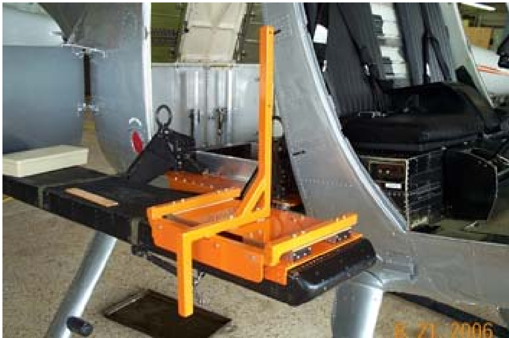
Figure 64. Manikin Roller Seat Assembly (Oblique, Installed).
