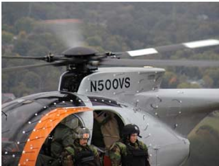
Figure 76. 50 Degree 8 Inch Deflector Flow Visualization Flight (Left Upper).
