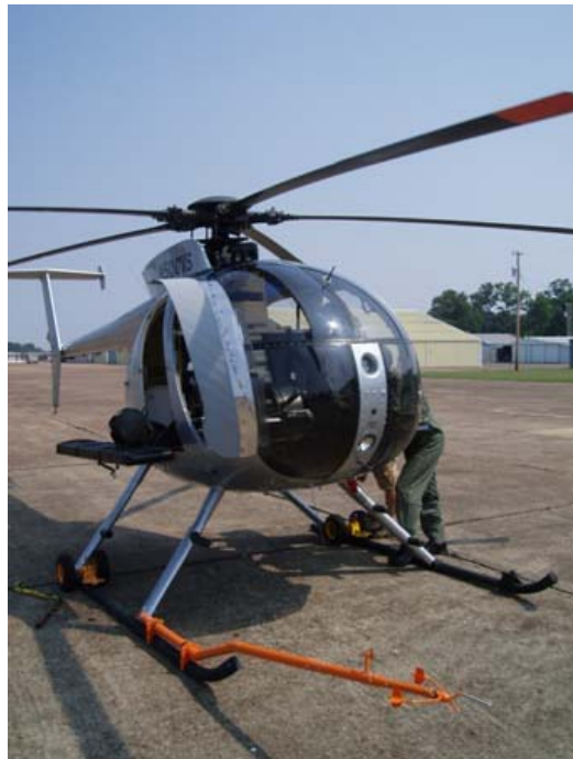
Figure 66. MD-500 Aircraft Configured for Deflector Flight.
