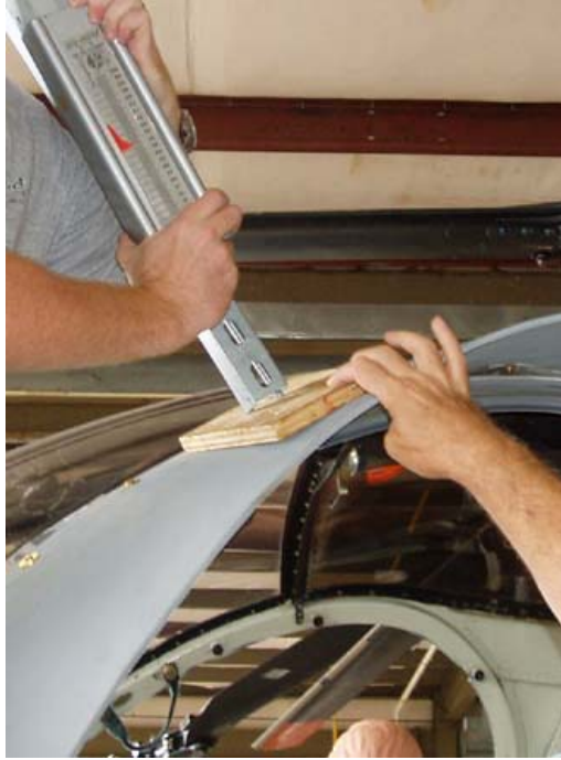
Figure 59. Static Load Testing of Installed Deflector (1).
