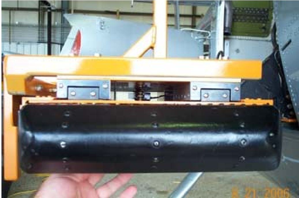
Figure 63. Manikin Roller Seat Assembly (Front, Installed).
