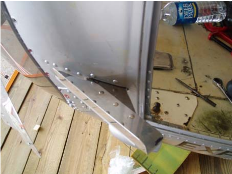
Figure 46. Lower Hinge Brace (Installed).
