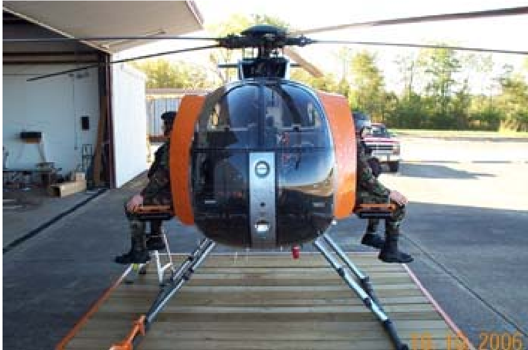
Figure 69. 40 Degree 8 Inch Deflector (Installed).
