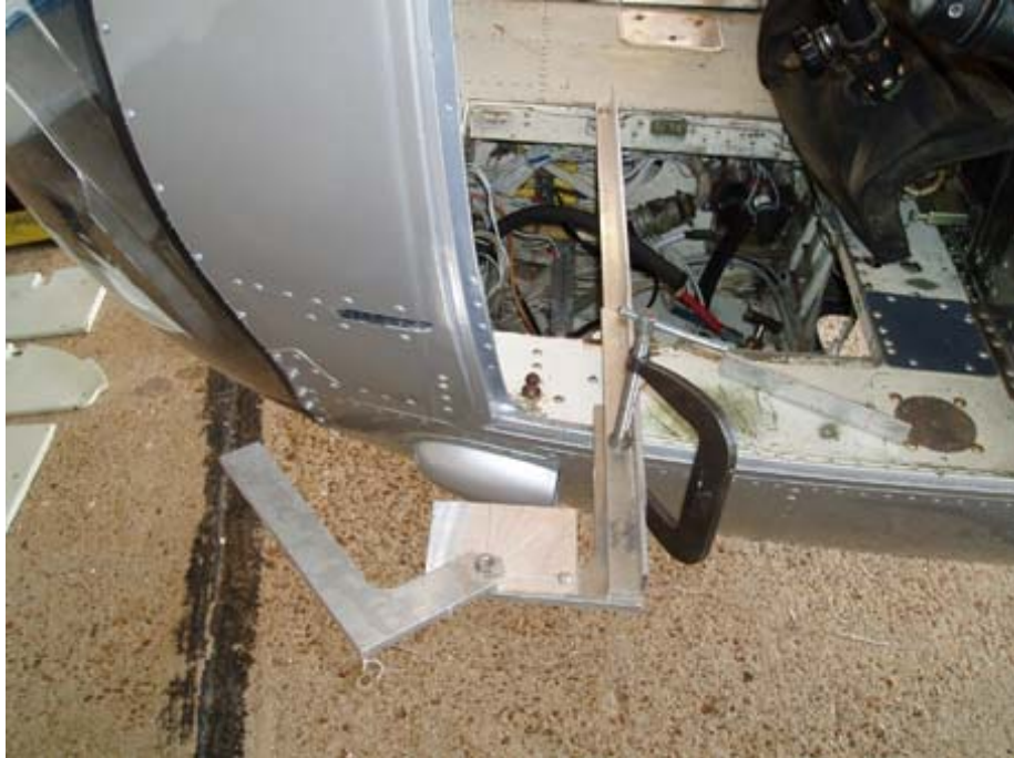
Figure 43. Fuselage Sweep Angle Measurement Protractor (Installed).
