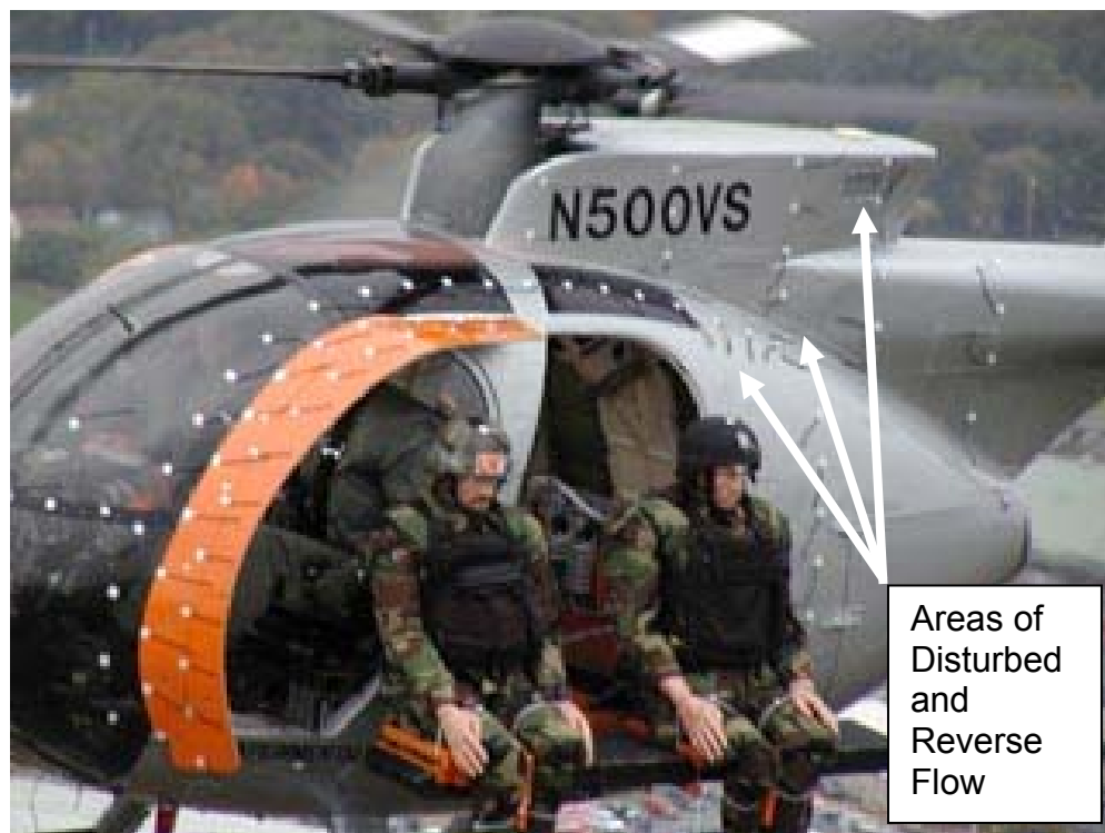
Figure 37. Airflow Visualization on Left Aft Fuselage.
