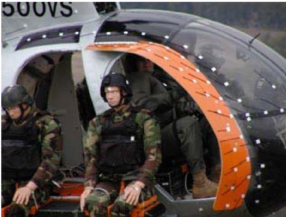
Figure 74. 50 Degree 8 Inch In-flight Flow Visualization (Right Close-Up).
