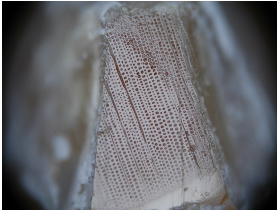
Figure 3-4. Loblolly pine cell wall after ultra-microtoming under optical microscope
