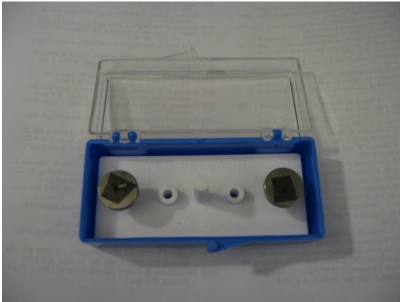
Figure 3-7. SEM stub and sample storage box
