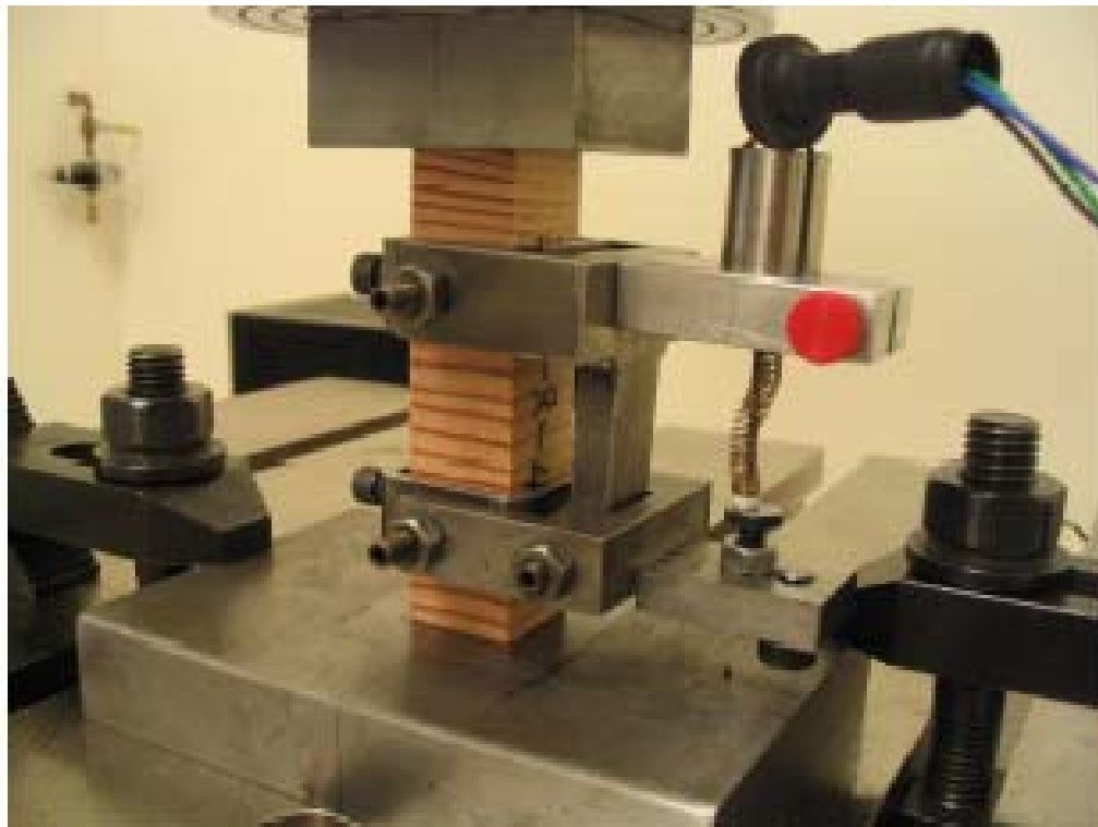
Figure 4-28. Macro scale wood compression test (Hong and Barrett, 2006)
