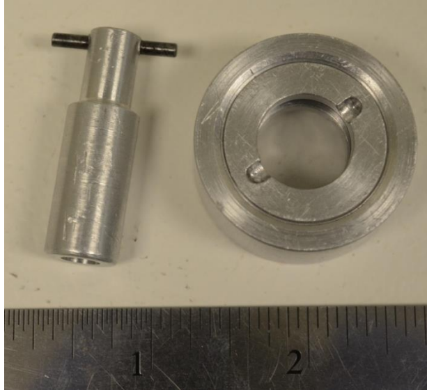
Figure 11: Sample holder (right) for transmission measurements and the tool for tightening it (left). The sample to be measured is protected by oil during the scan.
