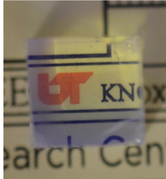
Figure 25: Full boule of CsCaBr 0.8 I 2.2 :Eu 2% (left) and a 1 cm cube sourced from the crystal.
