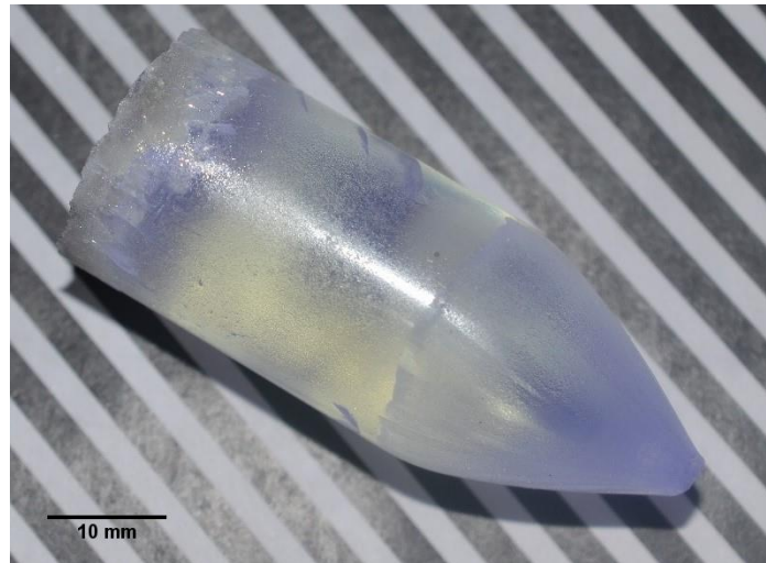
Figure 28: \varnothing 22 mm CsCaBr 0.8 I 2.2 :Eu crystal as removed from the growth ampoule. The rough surface texture is easily polished away.
