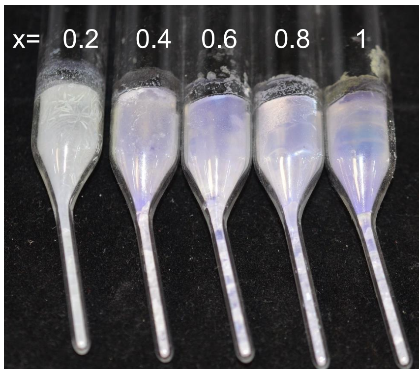
Figure 15: The five single crystal \text{CsCaBr}_{3-x}:\text{Eu} crystals still in growth ampoules.
