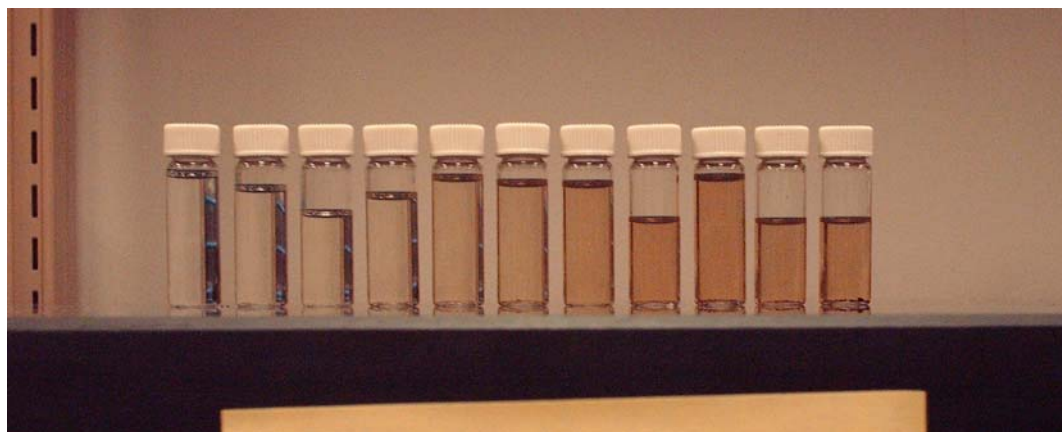
Figure 22. Acetonitrile Dilutions (1100:1) of (0 – 0.22 w/w) hydrolytic lignin.
