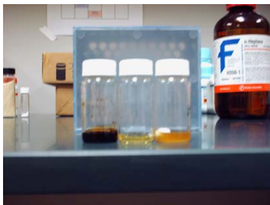
Figure 9. Solubilization of lignin, cellulose, and xylan in [Bmim][Cl], respectively.
