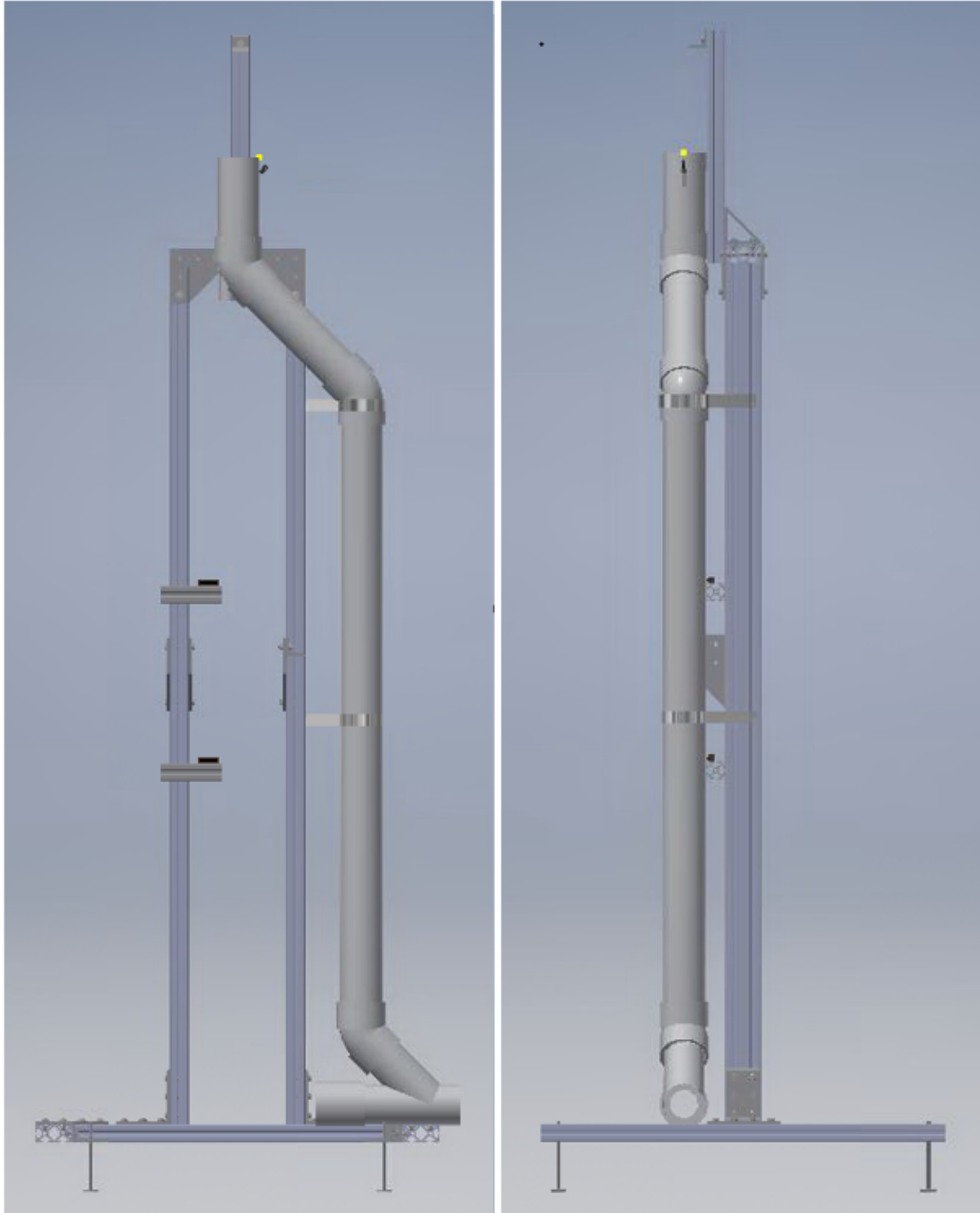
Figure 3.6. Rendering of the discharge system. The image on the left is a front view of the discharge system mounted to the stand, while the image on the right is a side view. Not shown is the 4" x 3" PVC closet bend, which is used to catch the flow leaving the Sample column and direct it into the discharge piping. This bend is connected to the lower branch of this 3" thin-wall PVC sewer pipe using a 3" flexible rubber coupling.
