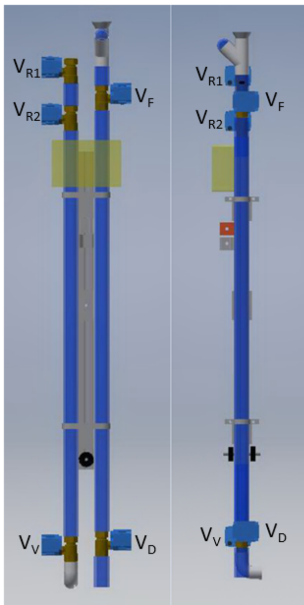
Figure 3.2. A rendering of the cylinder unit. The image on the left is a front view, with the Reference column on the left and the Sample column on the right. The image on the right represents a side view from the Sample cylinder side. V_{R1} and V_{R2} are the Top and Bottom Reservoir valves on the reference cylinder. The Vent valve on the reference cylinder is V_V . The Fill valve and the Drain valve on the sample cylinder are V_F and V_D , respectively.
