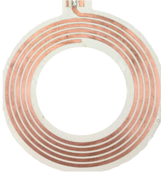
Figure 3.16: Self-resonant coil built with RO3003 for further reduced loss.
