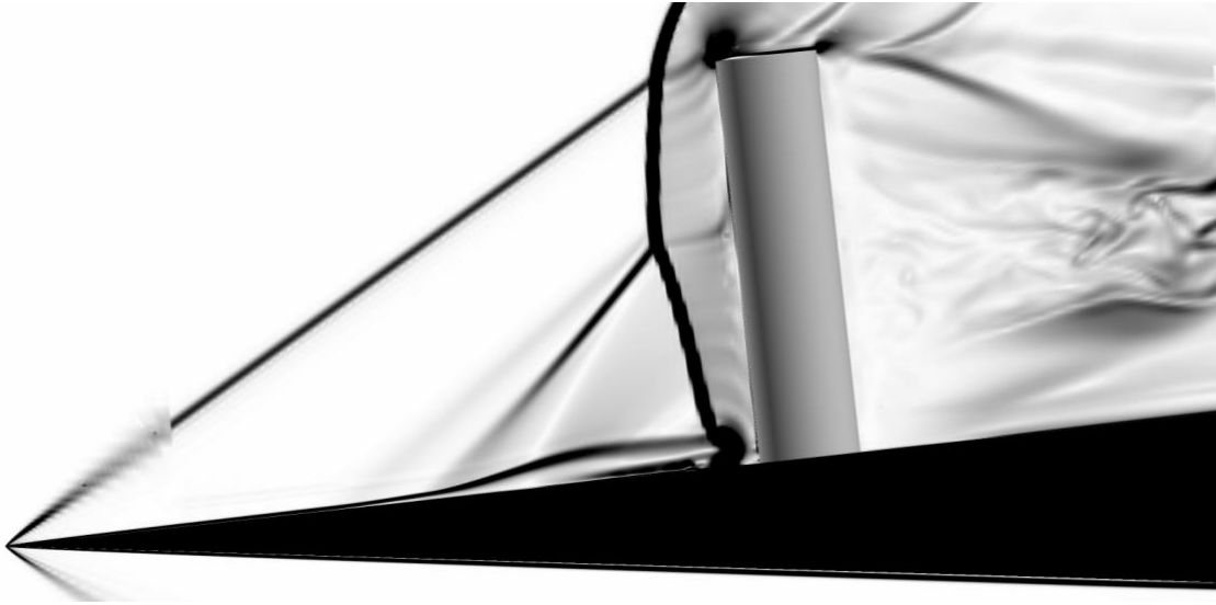
Figure 4.26 DDES-SA-QCR-AFT numerical Schlieren after reaching convergence. Flow is from left to right.
