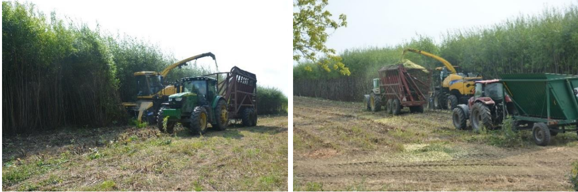
Figure 17. New Holland self-propelled forage harvester equipped with a woody coppice header and two collection equipment fleets consisting of a tractor towing a cane wagon were utilized for 2017 willow harvest.
