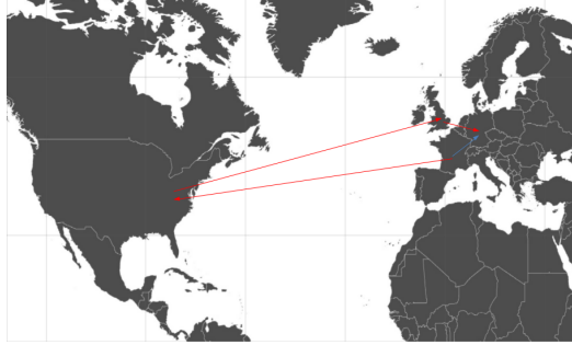
Figure 4.3: Visualizing of a geographically illogical path from France to Germany. This path is contained inside a single AS. Both the United States and the United Kingdom benefit from this path.
