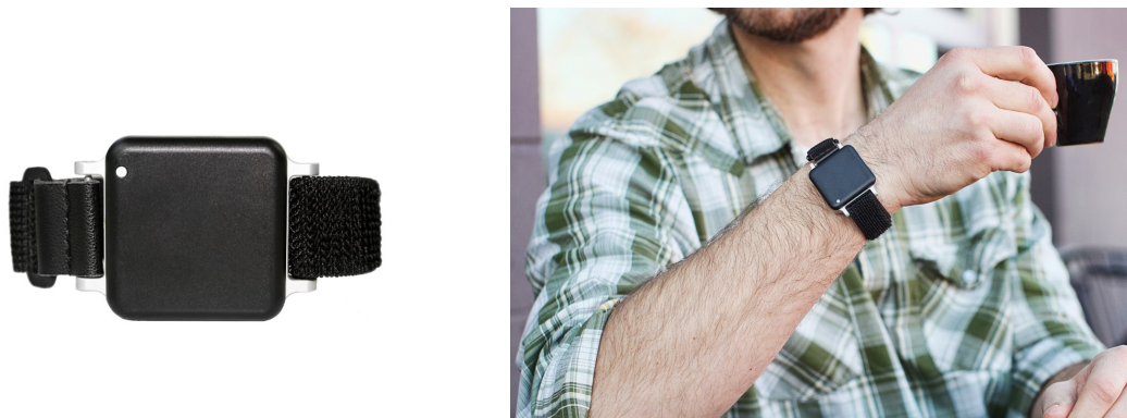
Figure 2.1: APDM Wearable Sensor for measuring linear acceleration and angular velocity [9][10]
