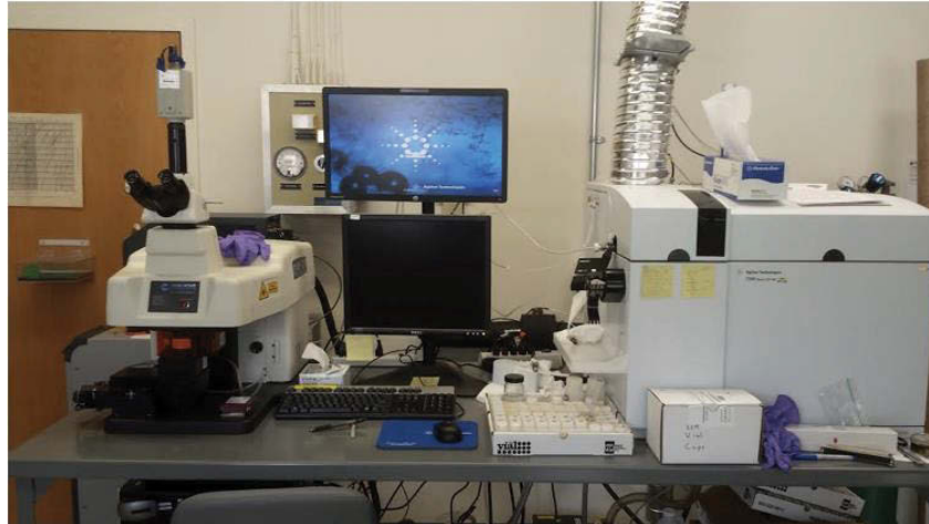
Figure 3.3 Assembly of the LA-ICP-CRC-QMS station at ORNL Stable Isotope Division with ESI UP-213nm YAG laser ablation unit on left and Agilent 7700x Quadrupole ICP-MS unit on right
