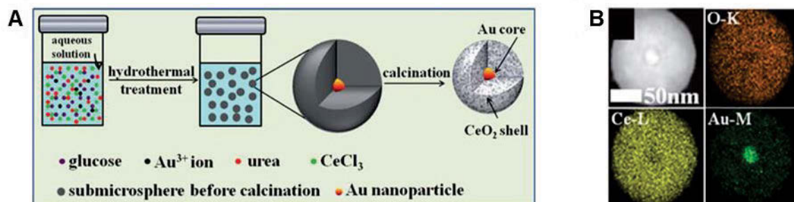
Figure 13. A) Synthesis of Au@CeO 2 core-shell structures and B) HAADF-STEM mapping image of one Au@CeO 2 heterostructure. Figure modified from reference. 75
