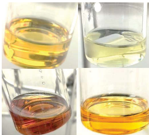
Figure 6. Ionic liquids used in this experiment. Top: [EMIM]Acetate (left), [EMIM]Formate (right). Bottom: [AMIM]Acetate (left), [AMIM]Formate (right).
