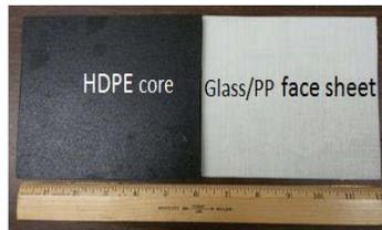
Figure 3.3 Image showing the front of glass/PP sheets and HDPE sheet used for the sandwich structure
