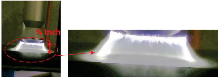
Figure 4.4 Plasma coming out from nozzle #22892 indicating large treatment area and varied plasms intensity within the treatment area
