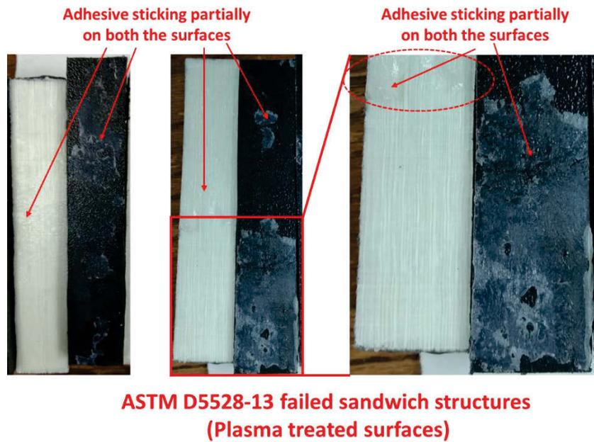
Figure A.19 Failed sandwich structure with plasma treatment to glass-PP and HDPE surfaces
