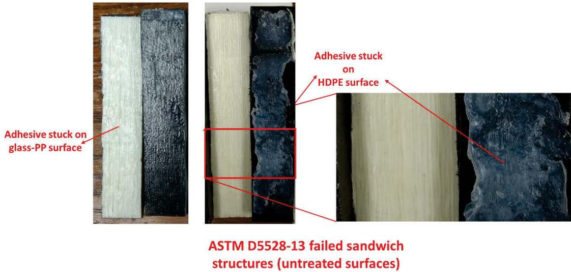
Figure A.18 Failed sandwich structure without surface treatment to glass-PP and HDPE surfaces
