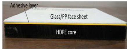
Figure 3.2 Image of the sandwich panel fabricated for the present study using glass/PP as face sheet and HDPE as core material
