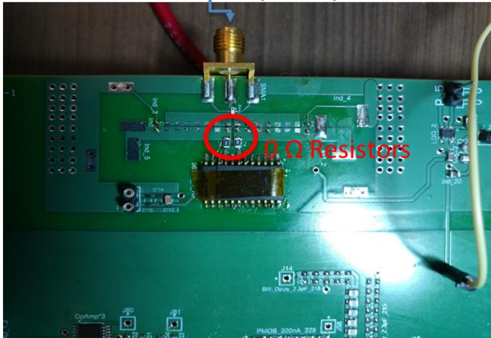
Fig. 5.33 The RF rectifier input impedance test set-up.
