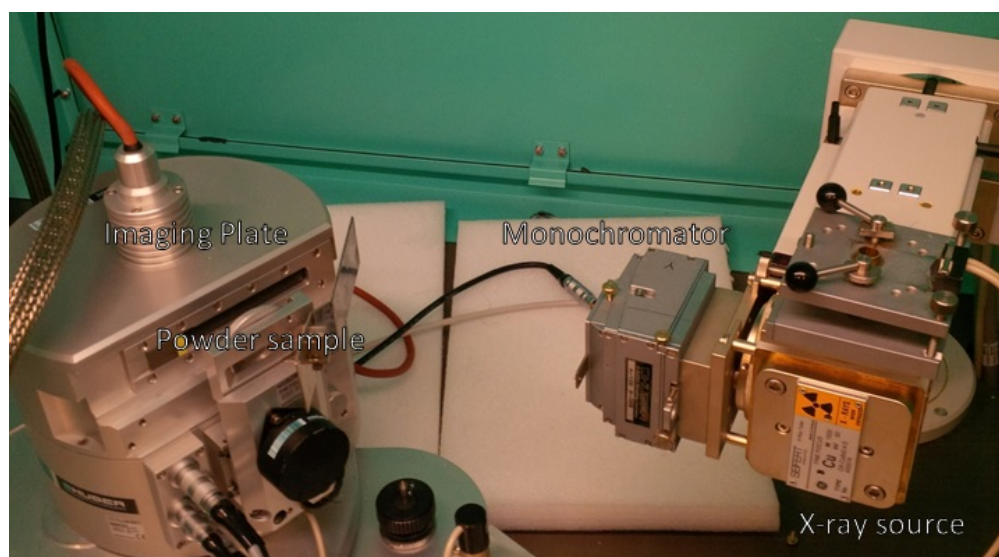
Figure 3.1: Labeled image of Huber X-ray Diffractometer showing the X-ray source tube with a copper anode, a monochromator to select the \text{Cu K}\alpha_1 wavelength, sample holder for the crushed powder sample, and imaging plate where the diffraction pattern is recorded.
