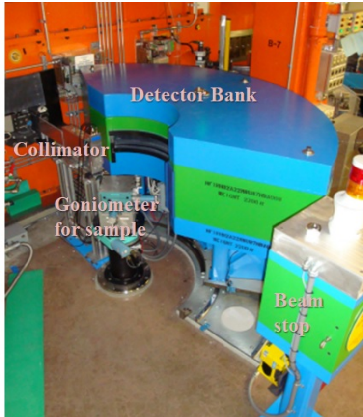
Figure 2.4: Image of HB-2A powder diffractometer located at Oak Ridge National Laboratory. The pre-sample collimator, detector bank of 44 He ^3 He detector tubes, goniometer for mounting sample environments, and the beam stop are labeled [46].
