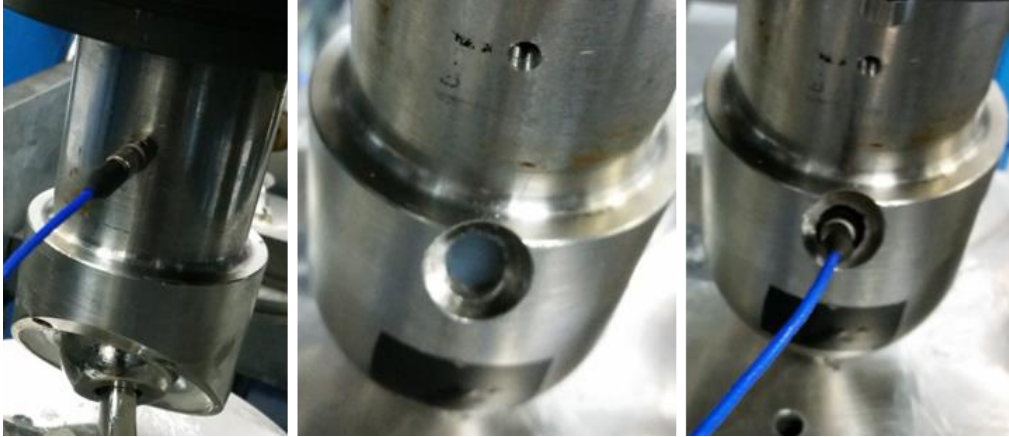
Figure 2.8. (Left) An accelerometer was screwed directly into the cup holder. (Middle) A tunnel was machined into the cup holder to expose the acetabular liner through the insertion hole present on the acetabular shell. (Right) An accelerometer was mounted directly to the acetabular liner.
