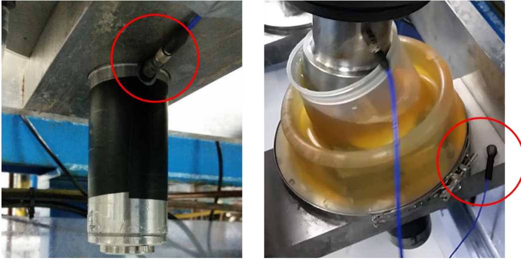
Figure 2.10. (Left) The “Femur ML” accelerometer was mounted below the simulator on the femoral stem holder such that its axial direction was medial/lateral. (Right) The “Femur SI” accelerometer was mounted on the cross beam of the femoral frame such that its axial direction was superior/inferior. A silicone gaiter was used to encapsulate the joint in a lubricant bath (diluted bovine serum).
