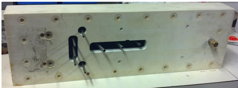
Figure 36. Tubing added to the bottom of the test article for blowing and dynamic pressure measurement.
