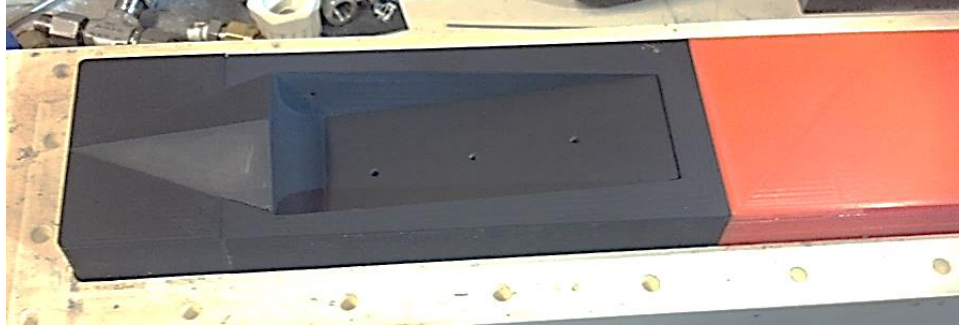
Figure 35. Test article assembled into the tunnel floorplate.
